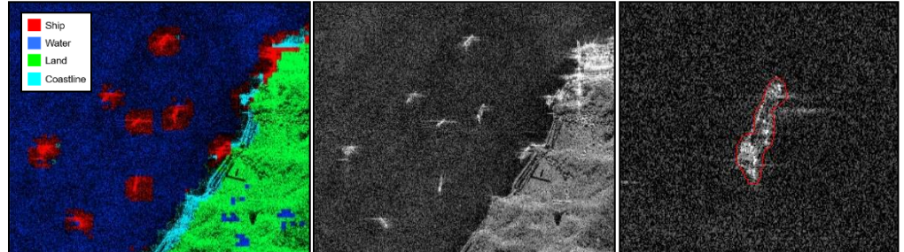
Convolutional neural network and heuristic ship detection techniques applied to commercial SAR data. Image source: © 2022 Capella Space Corp.
