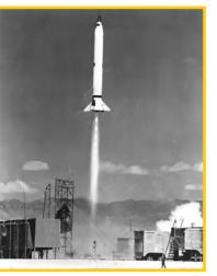
titude control provided by an NRL-designed gimbaled motor for steering and intermittent gas jets for stabilizing the vehicle after the main power cutoff. These attributes are now used extensively in large, steerable rockets and space vehicles. The Viking engine was one of the first large, liquid-propelled rocket engines produced in the U.S.
