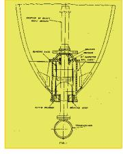
NRL's first effort was to develop an improved quartz-steel transducer. Extensive effort was placed on each of the components of the new sonar system, from the transducers and signal processing to the mechanical mounting and housing functions. Of particular significance was the development of the streamlined sonar dome to house the transducer. The dome enabled surface ships to make attacks at speeds up to 15 knots.
