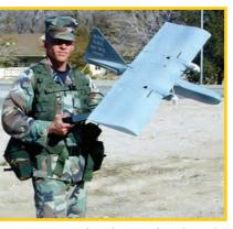
Name Corps Warfighting Laboratory, developed an affordable and expendable airborne sensor platform, Dragon Eye, to provide reconnaissance capabilities to small units of Marines to assess battle damage, to detect threats over the next hill or around the next building, and to prevent casualties from friendly fire. Dragon Eye went from a paper sketch to an operational system in 30 months. Prototype evaluation began in 2001. Production aircraft were deployed in Iraq and Afghanistan by 2004.
