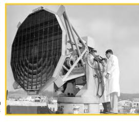
data directly into an IBM 709 computer, which, in turn, drove plotting boards in Central Control. In this manner, they tracked the launchings of the first U.S. space satellites, Explorer I and Vanguard I, at Cape Canaveral in 1958.
