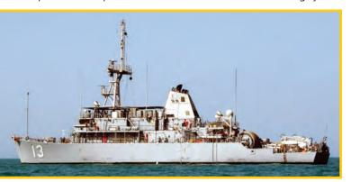
The USS *Dextrous* was relocated to the Persian Gulf, where the paint's solar reflective properties reduced heat buildup, increased crew comfort, and decreased the ship's infrared (IR) ship signature. LCA paint has been transitioned into the fleet, and now all Navy ships are painted with the NRL-designed paint.
