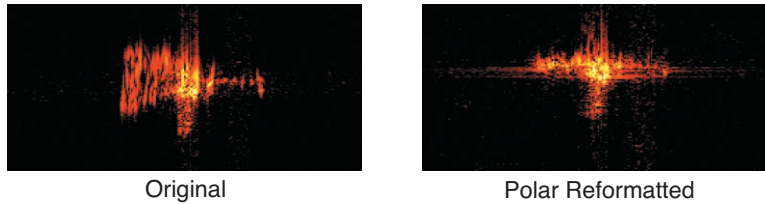
FIGURE 9 Example ISAR imagery showing the improvement in image quality using polar reformatting.
