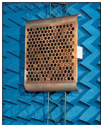
FIGURE 2 L-band phased array antenna with circular radiating elements (MIT Lincoln Laboratory development).
