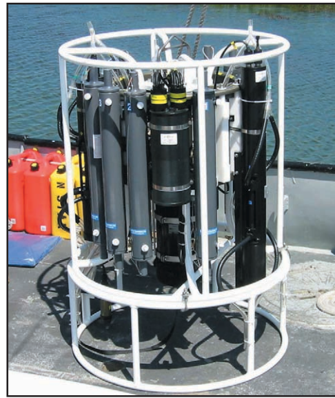
Profiling Optics and Water Return (POWR) system. White Seabird carousel frame protects underwater optical instruments (black cylinders) and water sample bottles (gray cylinders).
