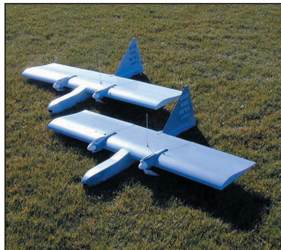
The U.S. Marine Corps Dragon Eye is an affordable, expendable airborne sensor platform for small unit reconnaissance and threat detection. The full-up system consists of a man-portable, 4.5-pound hand-launched air vehicle (shown) and a Ground Control Station to provide vehicle control and data retrieval.
