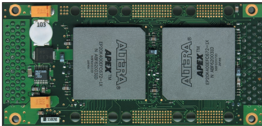
FIGURE 9 IP FPGA and processor interface hardware.
