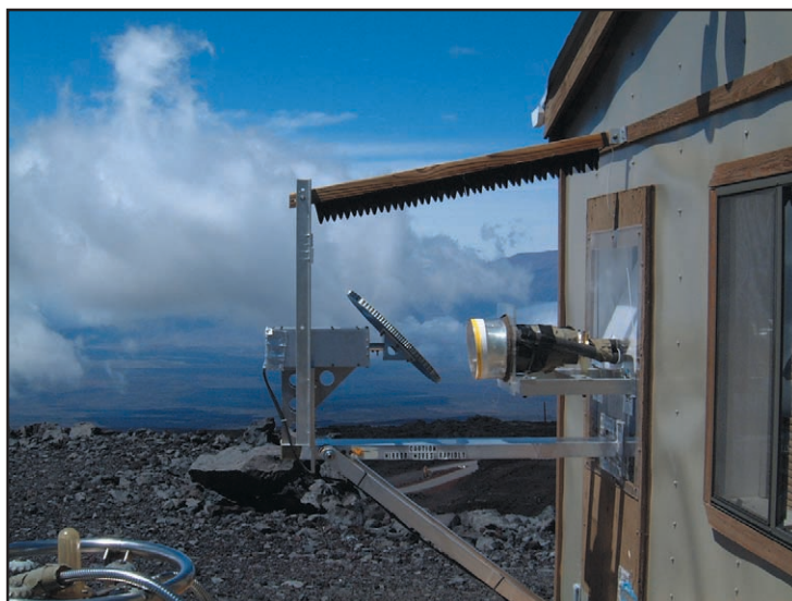
FIGURE 1 The WVMS instrument at Mauna Loa, Hawaii. The high altitude of this site makes it ideal for microwave measurements of the middle atmosphere.
