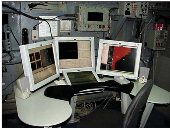
FIGURE 1 Single-operator sonar workstation deployed on USS Nicholson for the IUSW-21 sea test.
