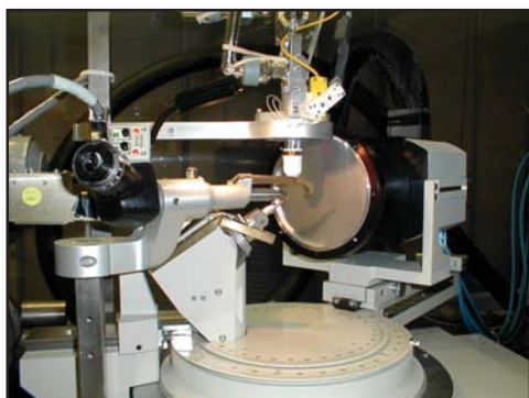
SMART 6000 CCD X-ray detector, which detects the X-ray scattering pattern of interest, is shown mounted on a platform goniometer. The scattering patterns are used to determine the geometric arrangements of molecules in their crystallographic form.
