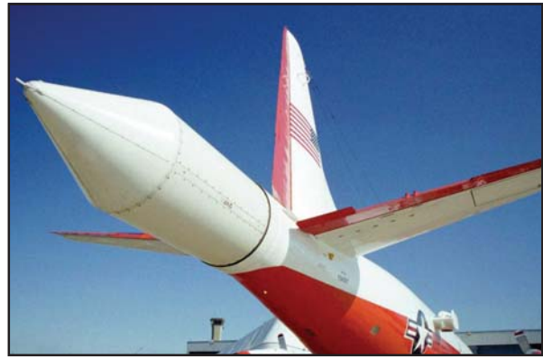
The Electra Doppler Radar (ELDORA) (located on the tail) and a laser (mounted to the side of the fuselage of Researcher 587) were used to collect atmospheric data in the skies over the midwest from the Bow Echo and Mesoscale Convective Vortices Experiment (BAMEX).
