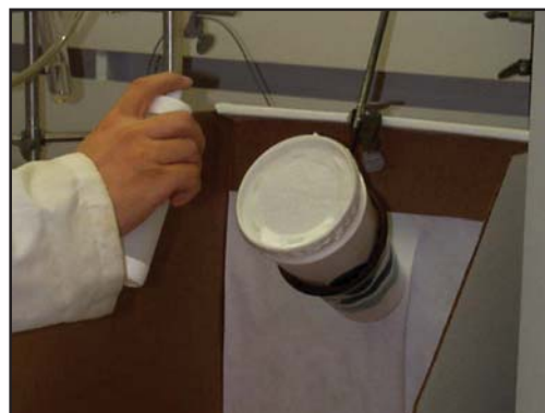
FIGURE 11 Fabrication of bioactive multilayers by spraycoating on cloth for individual protection.
