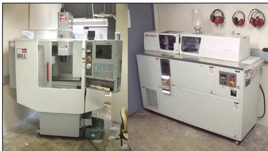
Plastic microfabrication facility with minimill and molding machine for high-resolution molding of plastic components used in biosensors.
