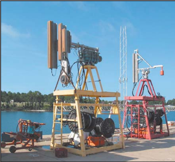
Broadband source array and receiving system being prepared for deployment. It is used by the High Frequency Acoustics Section to measure acoustic coherence links in very shallow water.
