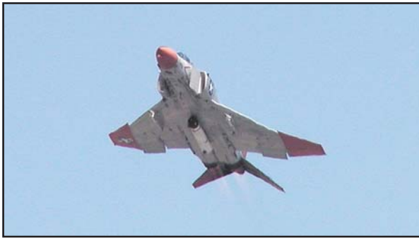
The NRL Tactical Directed Infrared Countermeasure (TADIRCM) system and the QF-4 drone aircraft on which TADIRCM was successfully live-fire tested. TADIRCM protects aircraft by detecting, tracking, and jamming heat-seeking anti-air missiles with infrared laser radiation.
