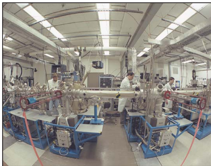
Molecular beam epitaxial growth of nanostructures using high vacuum, chamber-to-chamber sample transfer.
