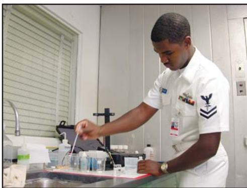
FIGURE 2 HM2 (SW) Clifton Butler (Naval Readiness Command, Mid-Atlantic) assists in testing the NACTEK protocols. The results from the colorimetric test are confirmed using a selective-ion electrode and test meter.
