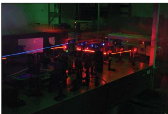
Femtosecond laser system for ultrafast dynamics; nonlinear mixing techniques are used to generate femtosecond pulses over a wide spectral range (mid infrared to deep ultraviolet) to investigate dynamic processes in molecules and materials. Recent studies include photochemistry and vibrational energy dynamics of ions in solution and in reverse micelles.
