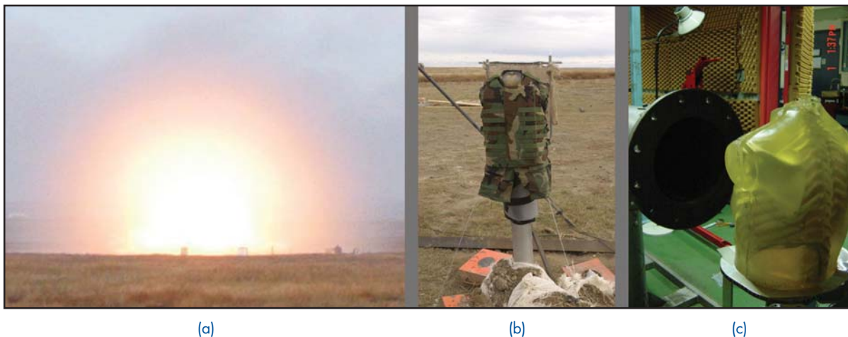
FIGURE 6 (a) Blast detonation at test sight. (b) Thoracic model with body armor at test sight. (c) Instrumented thoracic model undergoing shock impulse from pressurized shock tube.
