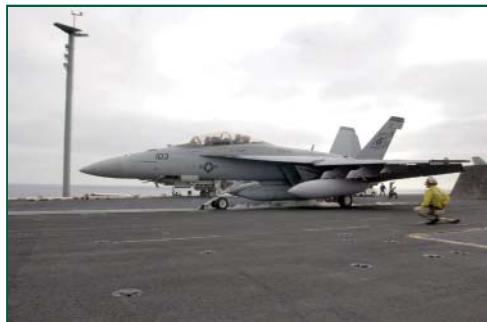
The shared reconnaissance pod (SHARP) on F-18F Super Hornet during trials.
