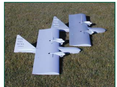
Dragon Eye – an expendable, man-portable, 5.5 lb, hand-launched air vehicle and a miniature Ground Control Station (GCS) to provide command and control and receive the aircraft's video and GPS position.
