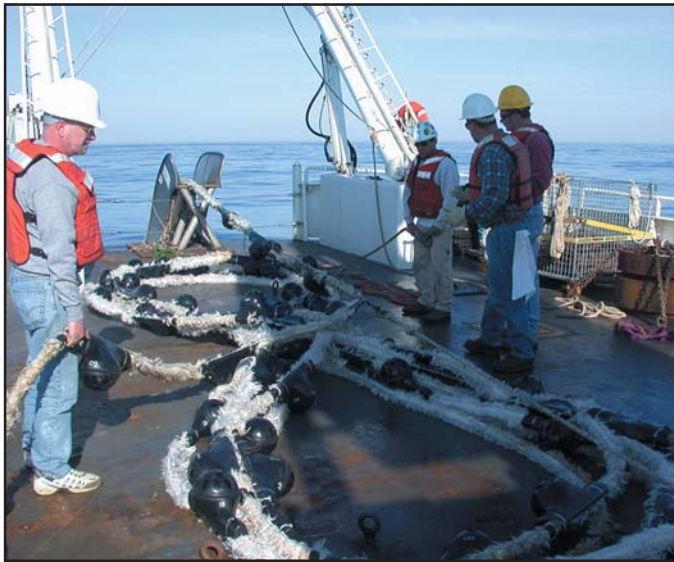
FIGURE 1 Deployment of the NRL 64-channel SRA from the stern of the R/V Endeavor during the TREX-03 time-reversal experiment.
