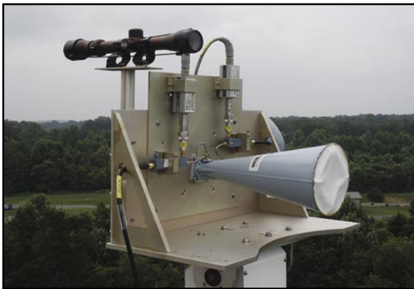
FIGURE 12 NIFTI horn assembly.
