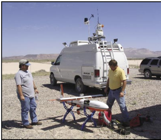
Mobile Ground Control Station (GCS) for unmanned vehicle research. The Mobile GCS is used for data analysis and provides communication and control to the unmanned vehicles during field experimentation. The photos show a typical field set-up and an internal view of the equipment van.
