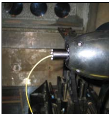
FIGURE 11 The downstream end of the propeller, showing the stationary side of the fiber optic rotary joint and the optical fiber carrying signals to the data acquisition system.
