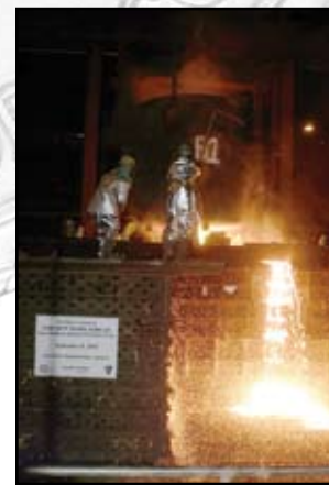
Workers from the Amite Louisiana foundry pour molten steel recycled from the World Trade Center into the mold of the bow stem of the Amphibious Transport Dock ship USS New York (LPD 21). About 24 tons of steel was salvaged from the World
