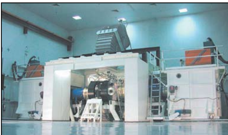
The NRL Electra system is used to develop high-energy high-repetition-rate KrF laser technology. The Electra 30-cm aperture electron-beam-pumped amplifier is shown in the photograph. A portion of the recirculating system that cools the laser gas can be seen at the top. This amplifier is capable of a 5 Hz repetition rate and has produced up to 700 J of laser light per pulse.
