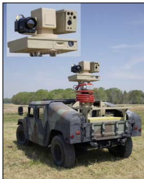
HMMWV installation of the Gunfire Detection and Location System that includes an IR detection sensor that automatically slews a day-night sensor suite to the position of hostile gunfire. The warfighter observes the scene and takes appropriate actions.
