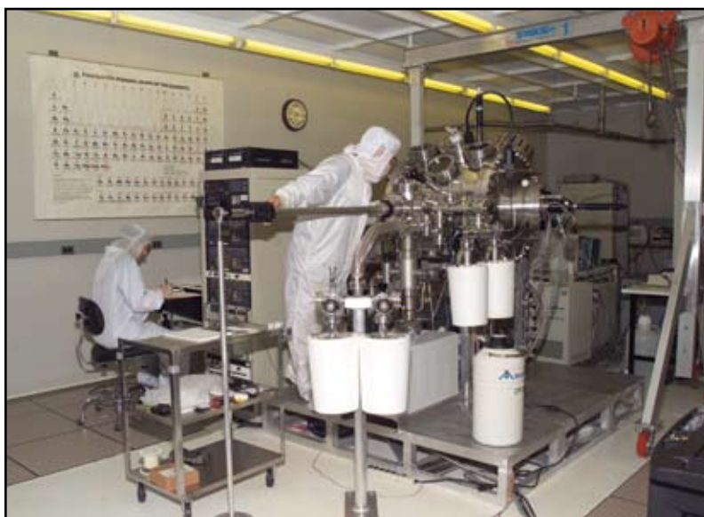
The Magnetoelectronics Fabrication Facility consists of a Class 1000 clean room facility equipped with tools for lithographic construction of magnetoelectronic and spintronic devices.
