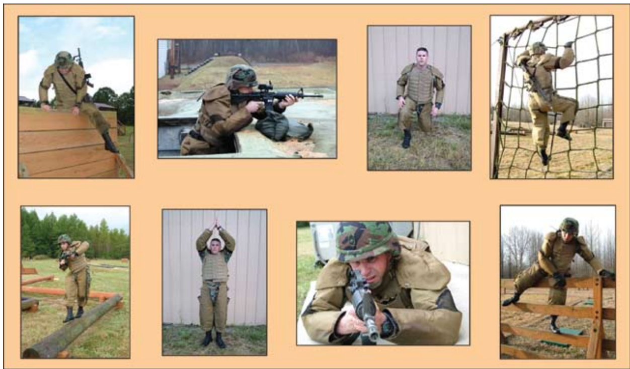
FIGURE 3 QuadGard testing by Army Research Laboratory at Aberdeen Test Center obstacle course and marksmanship range demonstrates the flexibility of the design and its compatability with existing body armor and infantry equipment.
