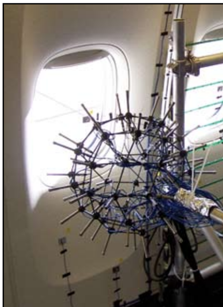
FIGURE 1 Fifty-element spherical array designed and constructed at NRL and mounted on a horizontal beam inside a Boeing 777 aircraft.
