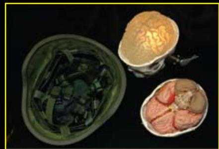
Surrogate materials and sensors are incorporated into the GelMan-Brain measurement systems to quantify headborne protective equipment performance with the aim of reducing traumatic brain injury.
