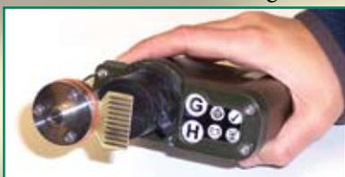
and explosives on more than 10 commercial and prototype detectors. CASPAR has the ability to selectively collect and concentrate the vapors of illicit substances due to its coating of NRL-developed sorbent polymer.
