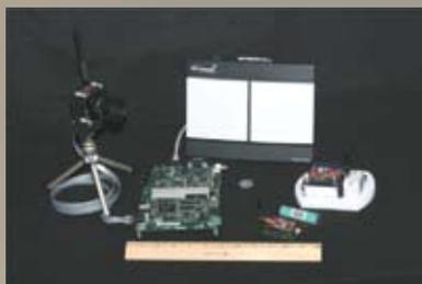
key technologies for the support of low-power unattended ground-based intelligence, surveillance, and reconnaissance (ISR) in remote locations. The heart of the system is the low-power embedded computer vision system that can track and identify targets while selecting imagery for near real-time up-link to any computer that has access to the Internet.
