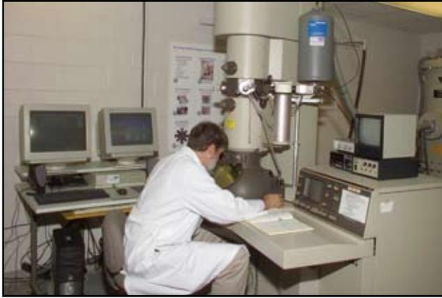
The Micro-Nano Structure Characterization Facility is capable of performing TEM, STEM, ARTEM, EELS, and Z-contrast imaging and spectral imaging.
