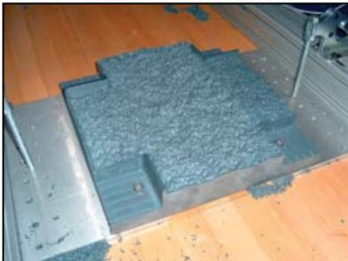
Fabrication of rough surfaces for acoustic analysis.
