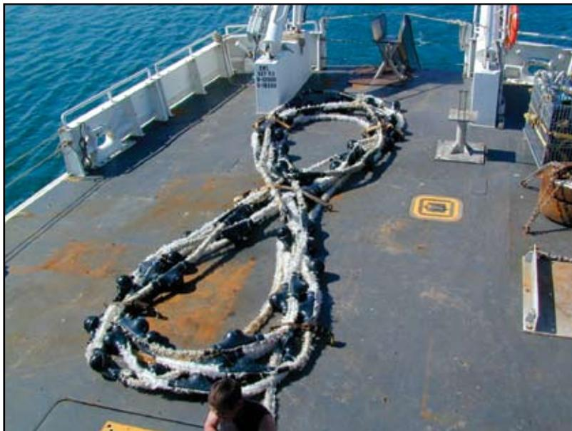
Source-receiver array for at-sea time-reversal experiments.
