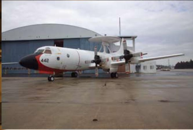
**NP-3D AEW with dome** – This P-3 at VX-1 is modified with the APS-145, or Hawkeye 2000, airborne early warning (AEW) system commonly found on the Navy E-2 Hawkeye aircraft. This system makes the aircraft ideal for airborne surveillance and cooperative engagements. The aircraft is currently used on a regular basis by the Missile Defense Agency in operations out of Hawaii.
