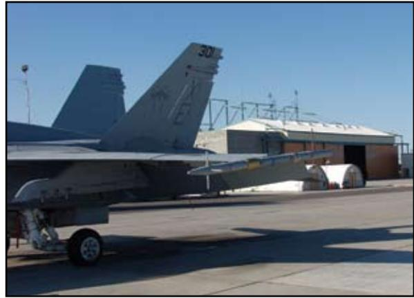
AN/ALQ-228(V)1 communications jamming pod.
