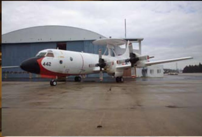
**NP-3D AEW with dome** – This P-3 at VX5-1 is modified with the APS-145, or Hawkeye 2000, airborne early warning (AEW) system commonly found on the Navy E-2 Hawkeye aircraft. This system makes the aircraft ideal for airborne surveillance and cooperative engagements. The aircraft is currently used on a regular basis by the Missile Defense Agency in operations out of Hawaii.
