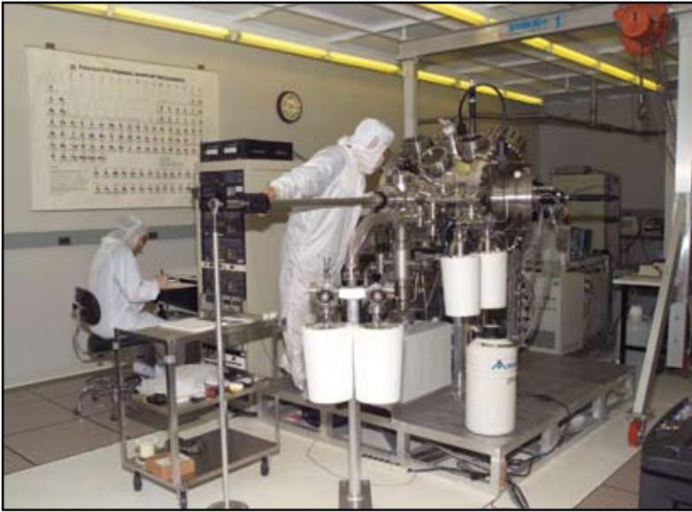
The Magnetolectronics Fabrication Facility consists of a Class 1000 clean room equipped with tools for lithographic construction of magnetolectronic and spintronic devices.
