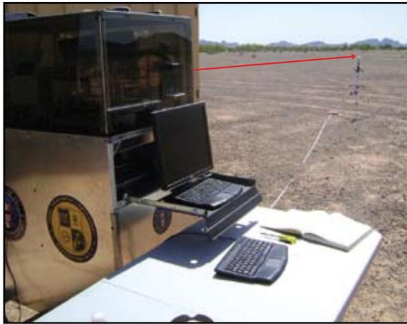
Field-testing the explosives detection system at Yuma Proving Ground, with the sample tripod at about 10 meters standoff. The red arrow illustrates the path of the invisible IR beam.
