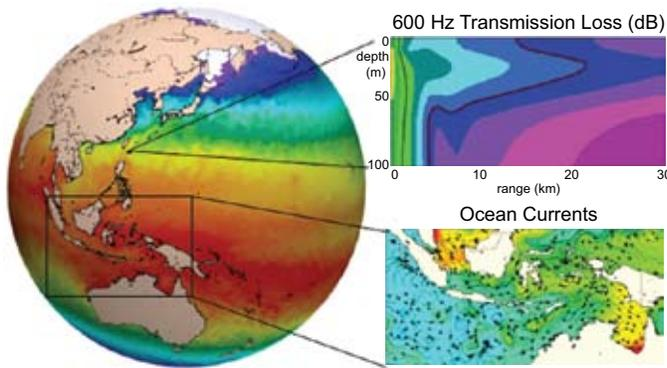
Transmission loss section from NOSSP using GOFS 2.6.
