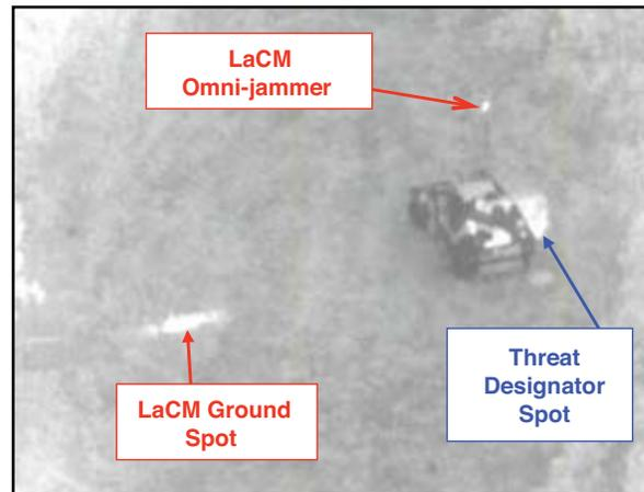
along with instrumented threat seekers installed on a test helicopter. This testing covered a wide range of backgrounds and attack geometries. A representative scene presented to the threat seekers is presented in the infrared image of Fig. 10. The center of the LaCM omni-jammer is seen as the small dot. The ground spot from the laser decoy lures the threat away from the HMMWV that is being illuminated by the threat's laser designator. During the testing, the LaCM was highly
