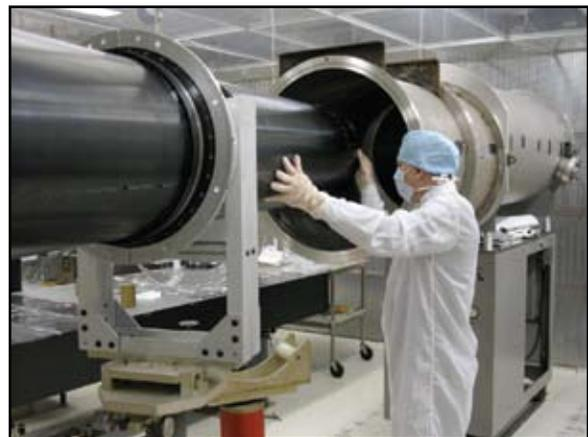
The VERIS payload is being loaded for testing into the Space Science Division solar rocket laboratory UV optical test chamber.
