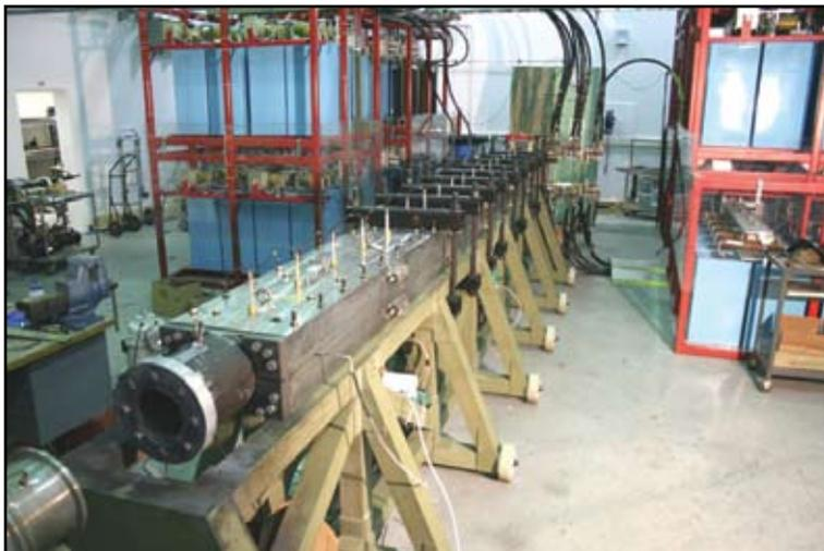
NRL's Materials Testing Facility railgun. The 6-m-long railgun is capable of launching 0.5-kG projectiles at 2.5 km/s using an 11 MJ capacitive energy store. This system is designed to perform experiments on bore materials under high-power launch conditions.
