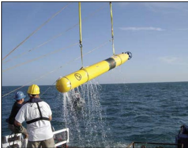
A 21-inch-diameter AUV is used for detection and classification in mine hunting and anti-submarine warfare applications.
