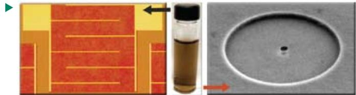
▶ Graphene, a single atomic sheet of graphite, has extraordinary physical properties, but its extreme thinness poses challenges in forming and manipulating it. In this work, we take advantage of a water soluble form of graphene in which oxygen functional groups are attached to the graphene basal plane.
