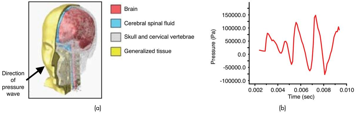
**FIGURE 1** (a) Finite element mesh of head. (b) Pressure profile on the face of the head from a 0.45 kg C4 charge exploded at 2.44 m from the head.
