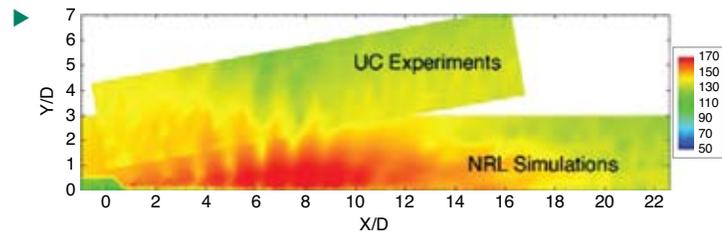
▶ The computed sound pressure level in the exhaust of supersonic military jet aircraft is compared to experimental data from the University of Cincinnati (UC). The agreement is excellent, indicating that the numerical simulations are very realistic.
