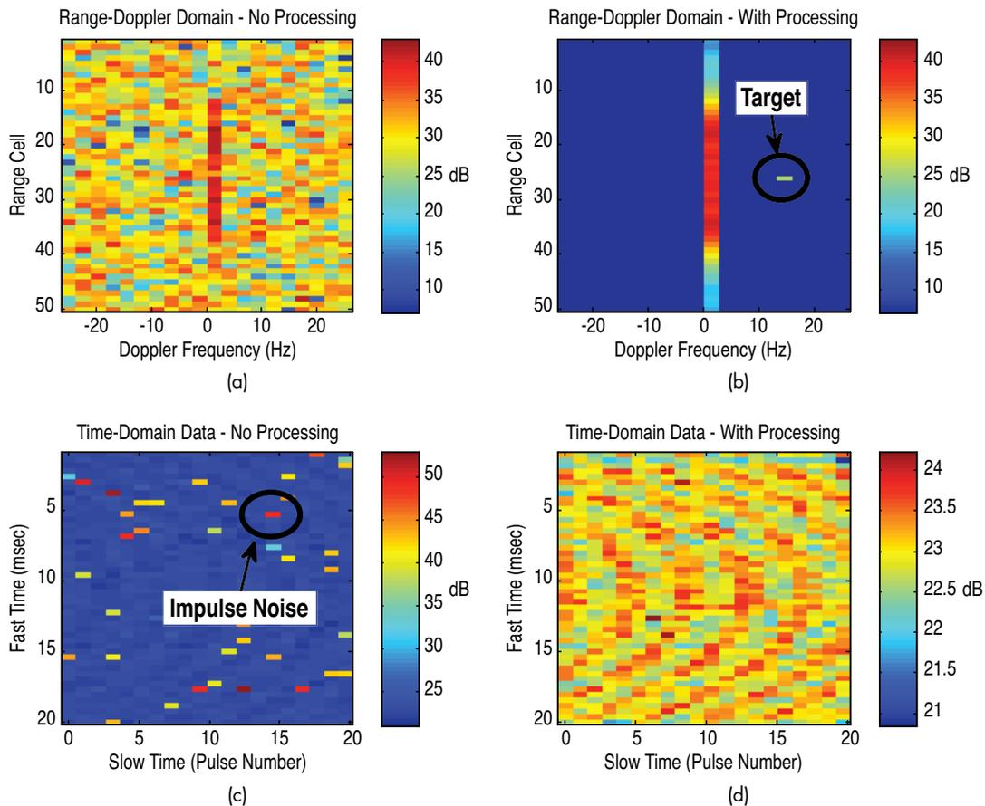
**FIGURE 13** Example of adaptive noise suppression technique operating on simulated data. (a) Range-Doppler image with no noise suppression processing; (b) time-domain representation of data, with impulsive noise present; (c) Range-Doppler image after impulsive noise suppression, target can be detected; (d) time-domain data after impulsive noise has been filtered.
