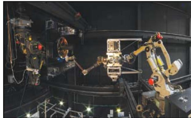
Full-scale spacecraft rendezvous and docking testing in NRL's Proximity Operations Laboratory against a simulated geosynchronous communication satellite (left). Spaceflight-ready two-meter robot arm (center).
