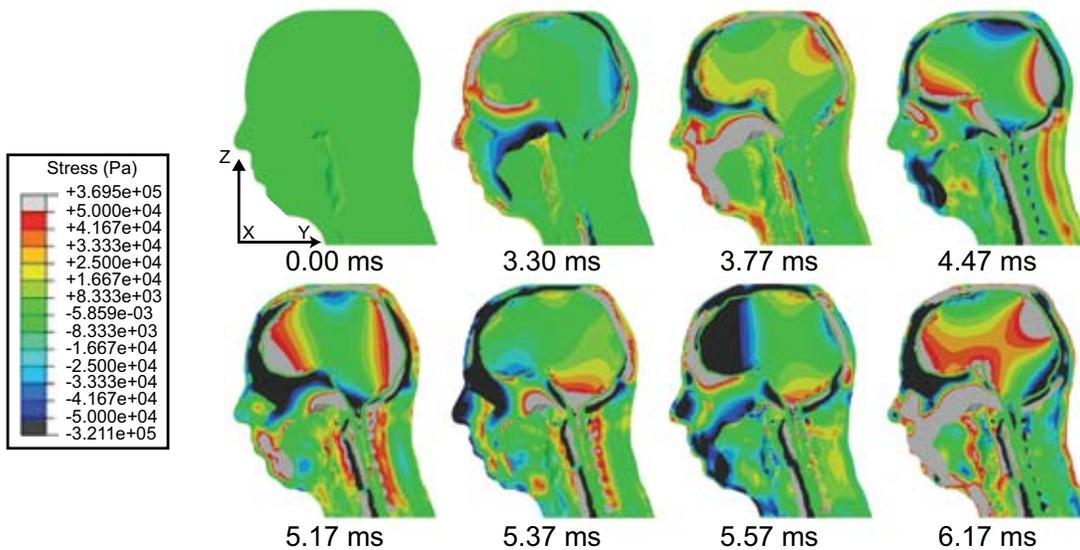
**FIGURE 2** Pressure contours in the head at the sagittal plane.
