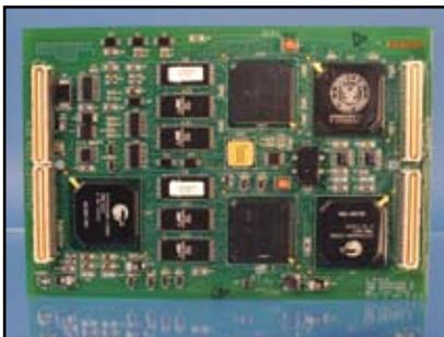
The PEIP-II multi-channel software programmable MILS (multiple independent levels of security) cryptographic module.
