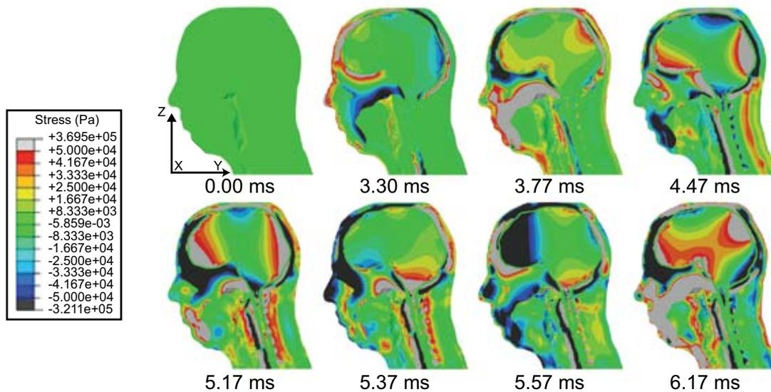
**FIGURE 2** Pressure contours in the head at the sagittal plane.
