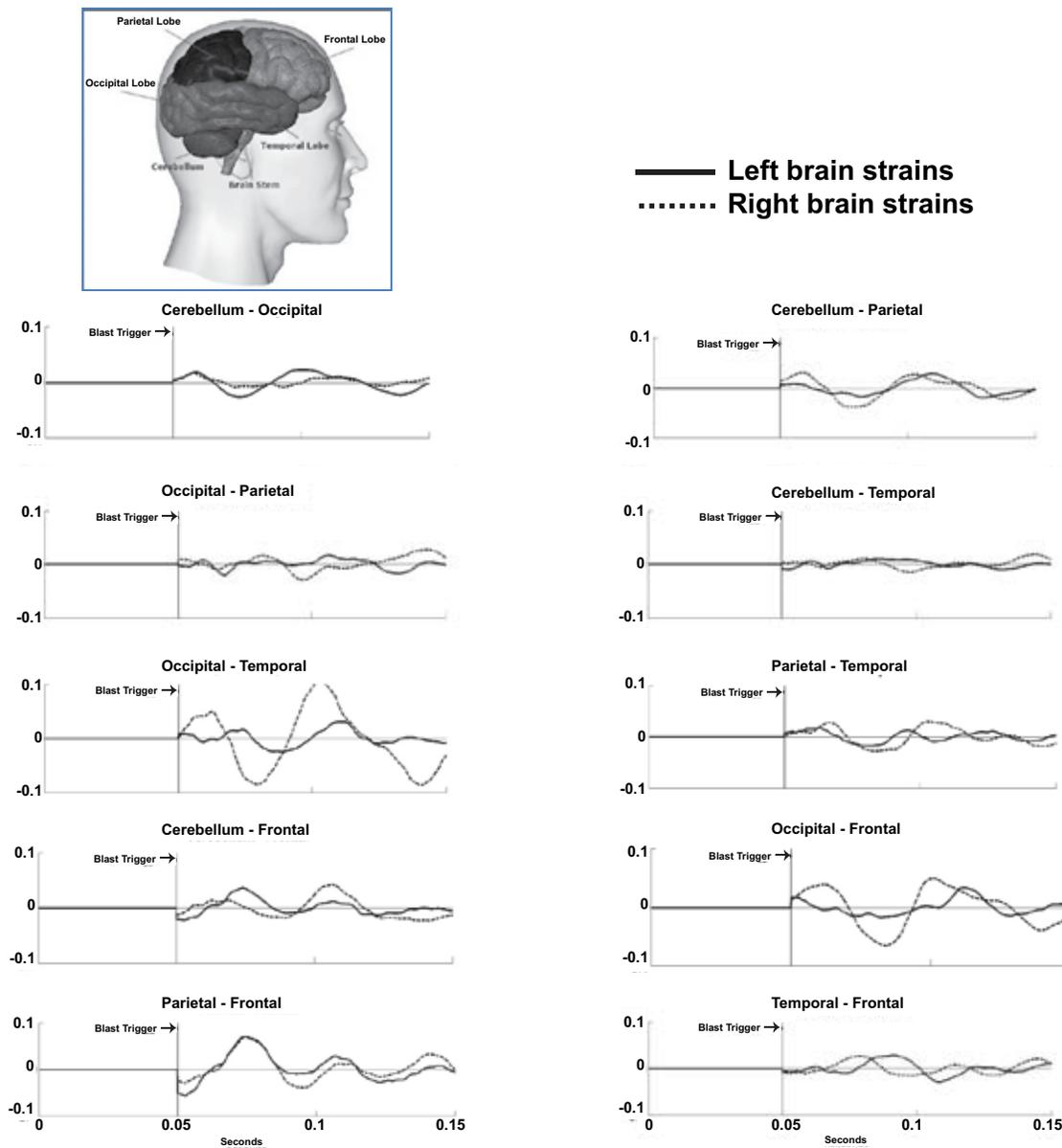
**FIGURE 4** Calculated strain response from accelerometers in the brain from a C4 charge exploded at distance of 2.44 m from HSB.
