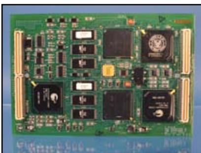
The PEIP-II multi-channel software programmable MILS (multiple independent levels of security) cryptographic module.
