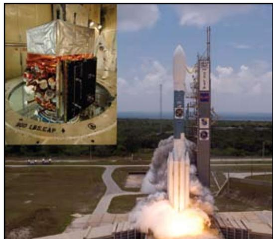
Launch of NASA's Fermi Gamma-ray Space Telescope from Cape Canaveral Air Force Station. Inset: The Fermi spacecraft during installation on the Delta IIIH rocket. The LAT instrument is the large silver rectangular instrument on top of the spacecraft.
