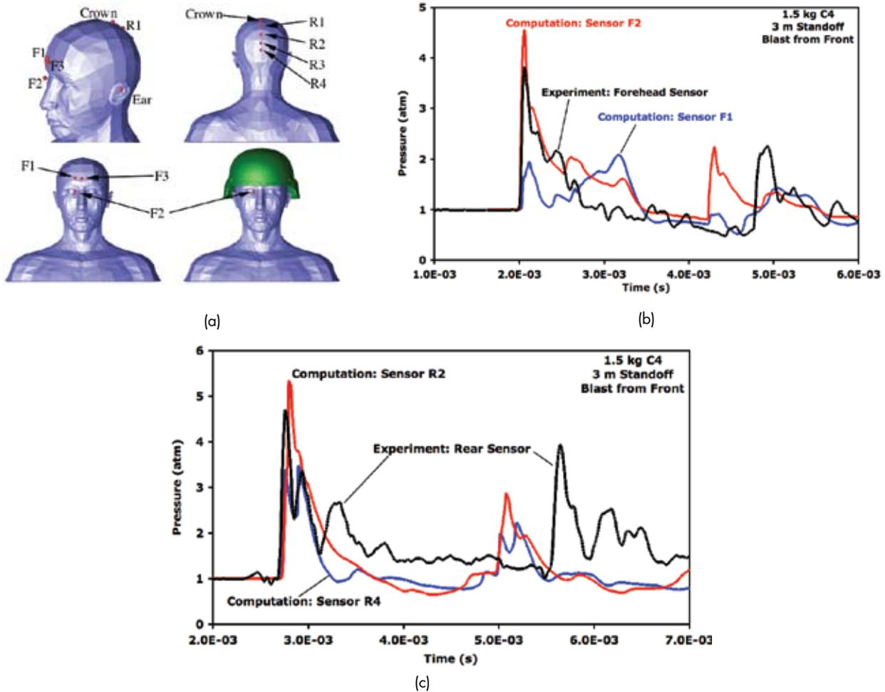
**FIGURE 5** (a) Sensor locations for the computational data. (b) Forehead pressure traces for the forward blast scenario. (c) Rear pressure traces for the forward blast scenario.
