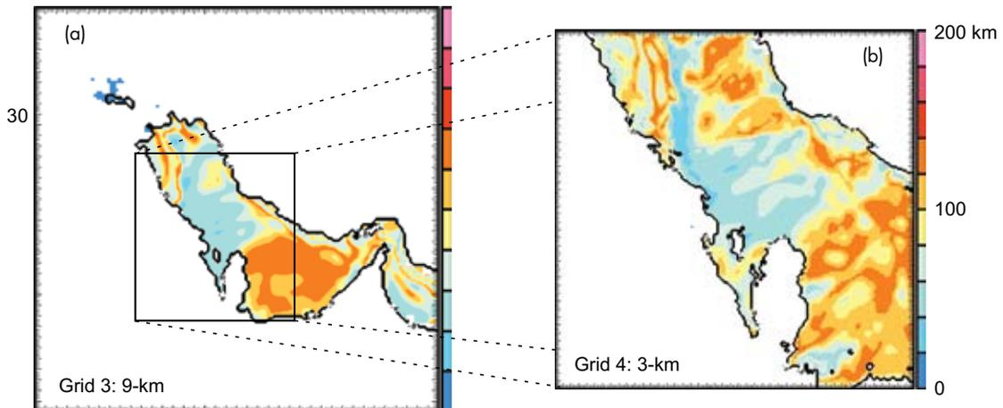
**FIGURE 2** Comparison of the radar performance surface for an X-band shipboard radar showing maximum detection range (km) for a 90% POD of a small surface target from COAMPS 9-km resolution fields (a) and 3-km resolution fields (b).
