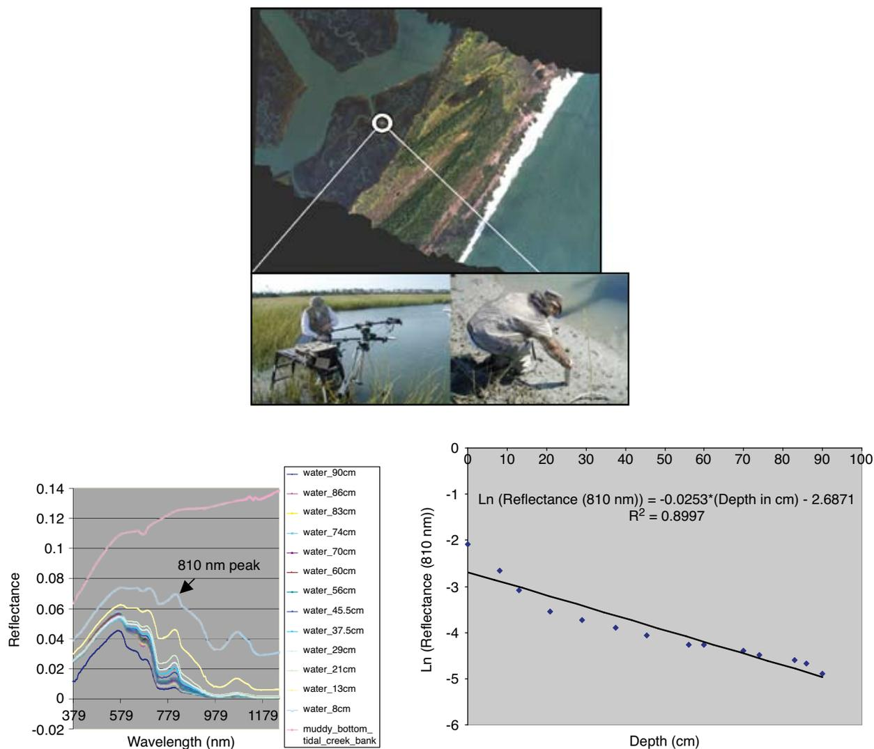
**FIGURE 9** Top: In situ spectrometry site on salt marsh tidal creek bank with muddy bottom, at high and low tide, Parramore Island, VA. Bottom left: In situ spectral reflectance vs depth profiles. Bottom right: Regression at the 810 nm feature.
