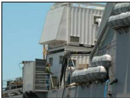
Multifunction Electronic Warfare (MFEW) above- and below-deck trailers and receive array installed on USS Comstock.
