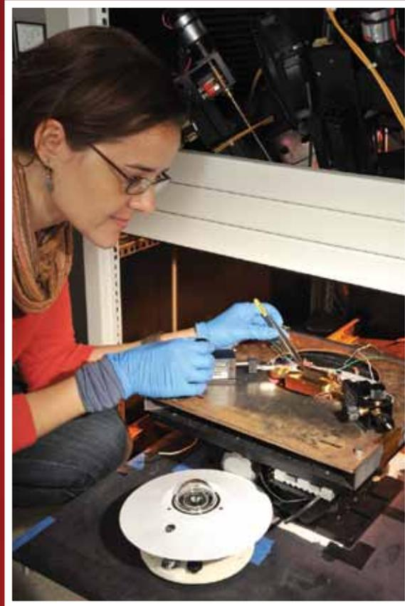
A scientist takes current–voltage (I–V) measurements under a triple source AM0 and AM1.5G calibrated solar simulator as part of advanced photovoltaics research. (AM0, or Air Mass Zero, refers to the solar spectrum in space, and AM1.5 to the solar spectrum on Earth.)
