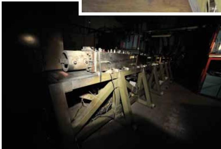
*The Materials Testing Facility railgun focuses on materials issues for a major Navy effort to develop a long-range, electromagnetic launcher for a future electric ship. The NRL Plasma Physics Division conducts a broad program in laboratory and space plasma physics and related disciplines, high power lasers, pulsed-power sources, intense particle beams, advanced radiation sources, materials processing, and nonlinear dynamics.*
