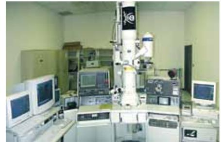
The JEOL JEM-3010 transmission electron microscope.
