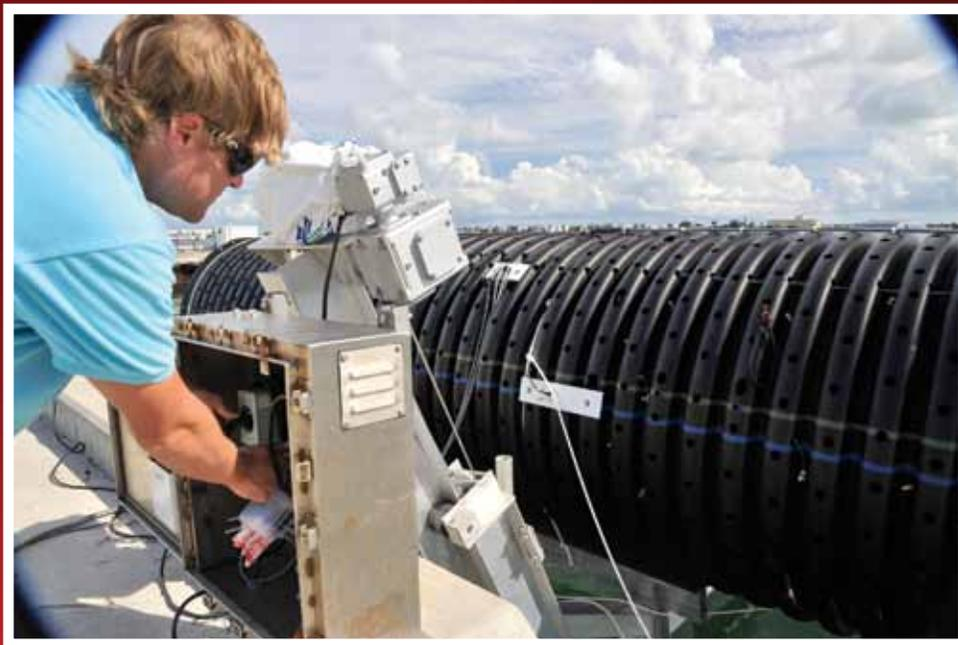
Cathodic protection design: NRL has a physical scale modeling facility to construct detailed physical models of ship and submarine hulls that are outfitted with sensors, materials, and control systems to model corrosion protection systems and the resultant electromagnetic signatures.
