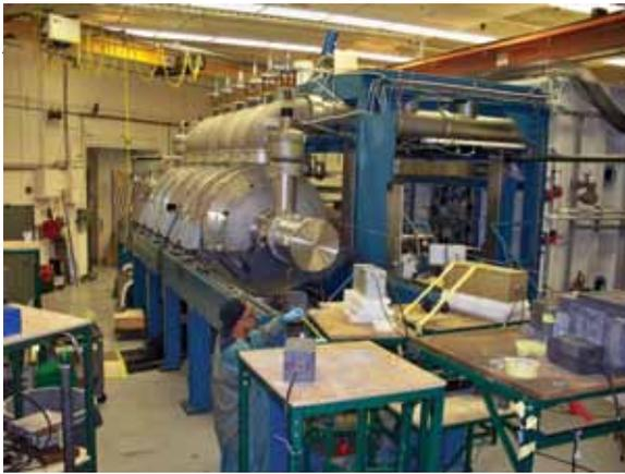
A technician aligns an array of specialized X-ray, gamma-ray, and neutron diagnostics to characterize the radiation output of the Mercury pulsed power generator in preparation for active detection experiments.
