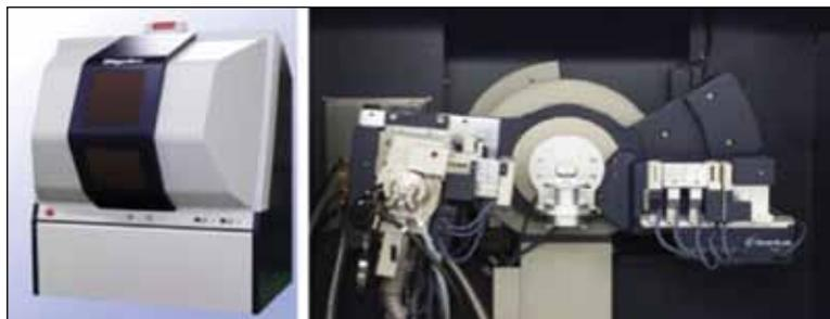
Chemistry Division's new multipurpose X-ray diffraction system is capable of a range of wide angle and small angle x-ray measurements. SmartLab exterior (left, 4 ft × 4 ft × 5 ft) and interior (right) views.
