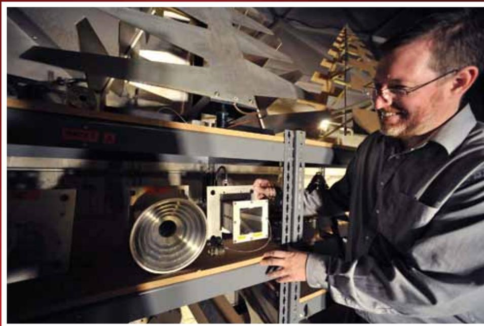
An employee of the Space Systems Development Department points out some of the many antenna feeds used on the 18 meter antennas at NRL's Midway Research Center. These customized feeds are quickly interchanged and are used by a variety of clients on these antennas depending on the transmit or receive test being conducted (250 MHz to 18 GHz).
