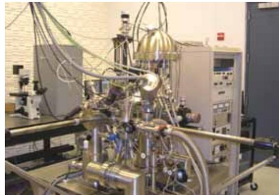
The Optical Sciences Surface Characterization Facility includes instrumentation for ultraviolet and X-ray photoemission spectroscopy (UPS and XPS), atomic force microscopy (AFM) and scanning tunneling microscopy (STM), and STM-induced light emission (STM-LE) measurements.
