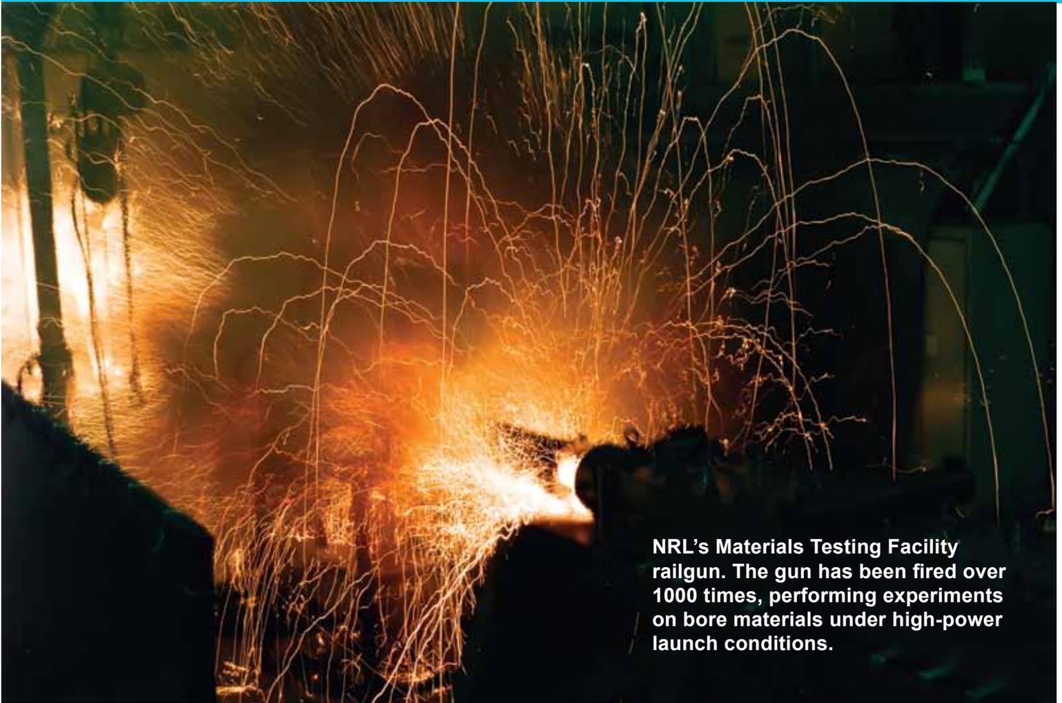
**NRL's Materials Testing Facility railgun. The gun has been fired over 1000 times, performing experiments on bore materials under high-power launch conditions.**
