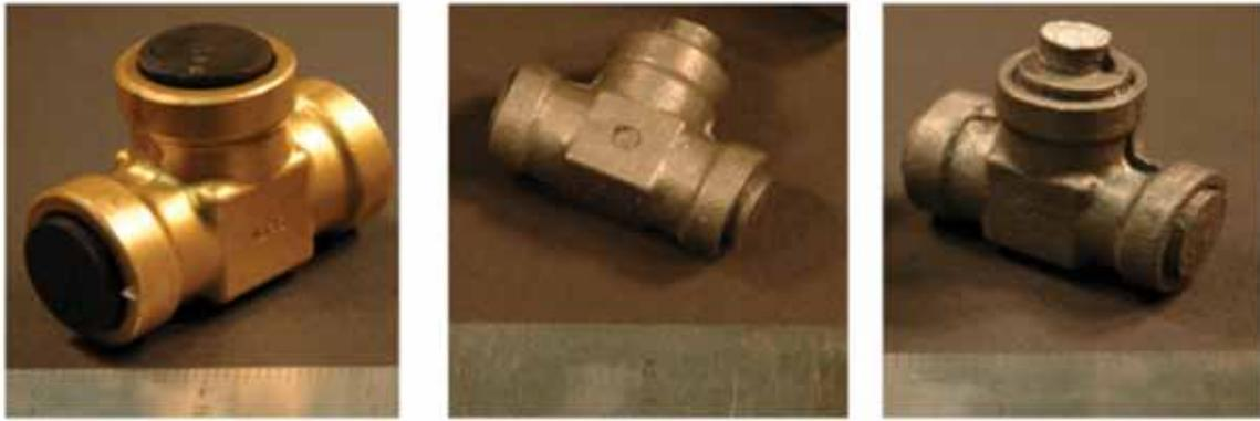
Left to right: original brass valve; unprocessed Ti powder compact having the same shape; and sintered Ti compact.
