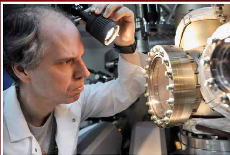
An employee of the Electronics Science and Technology Division prepares to transfer a sample in a molecular beam epitaxy system for the growth of compound semiconductors.
