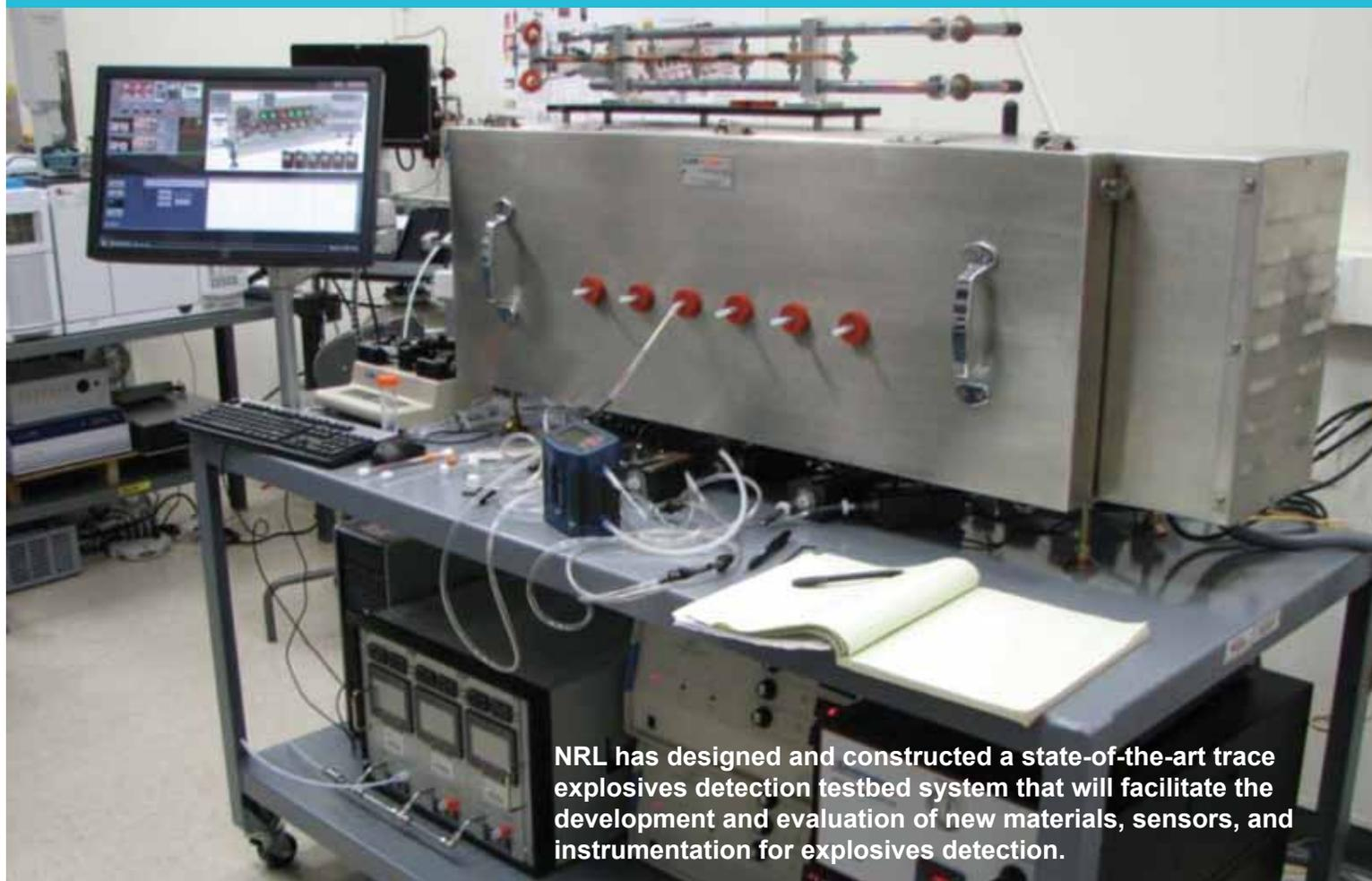
**NRL has designed and constructed a state-of-the-art trace explosives detection testbed system that will facilitate the development and evaluation of new materials, sensors, and instrumentation for explosives detection.**
