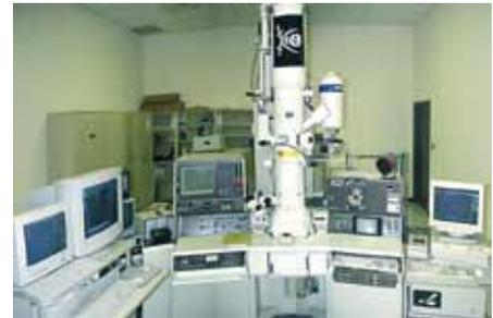
The JEOL JEM-3010 transmission electron microscope.
