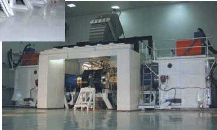
Electra repetitively pulsed krypton fluoride (KrF) laser. Potential applications of this laser and electron beam technology include inertial fusion energy, materials modification, and environmental remediation.
