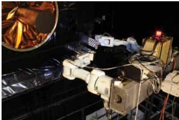
A robotic servicer is preparing to autonomously release a snagged array on a geosynchronous satellite mockup. The right servicing arm is initiating insertion of its fiducial tool into the laser-detected gap between the snagged array and the main satellite bus, guided solely by a camera imaging the scene from the left arm.
