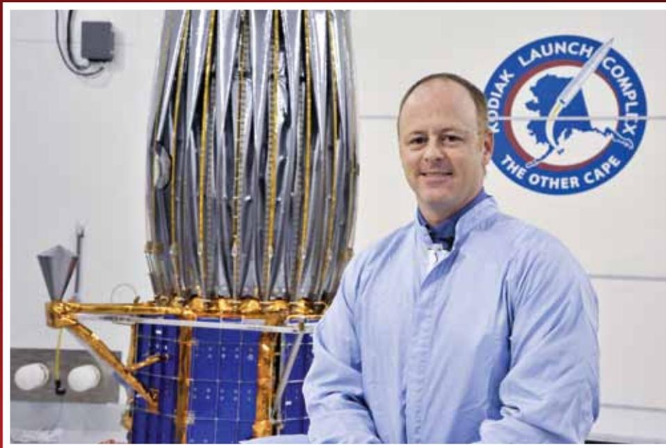
A program manager for the TacSat-4 satellite stands next to the spacecraft at the Alaska Aerospace Kodiak Launch complex, Alaska. TacSat-4 was launched September 2011 aboard an Orbital Sciences Minotaur-IV launch vehicle into a highly elliptical orbit (HEO) with an apogee of 12,050 km.
