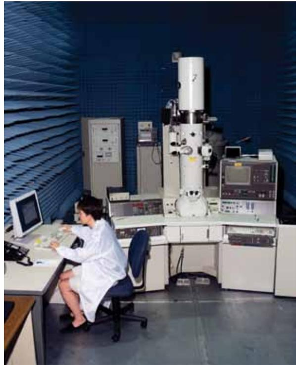
Transmission electron microscopy.
