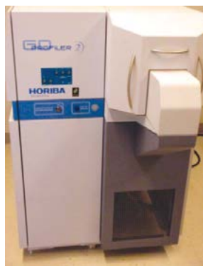
The Division's new Glow Discharge – Optical Emission Spectrometer performs high precision elemental analyses and correlates these elemental analyses with depth profiles.
