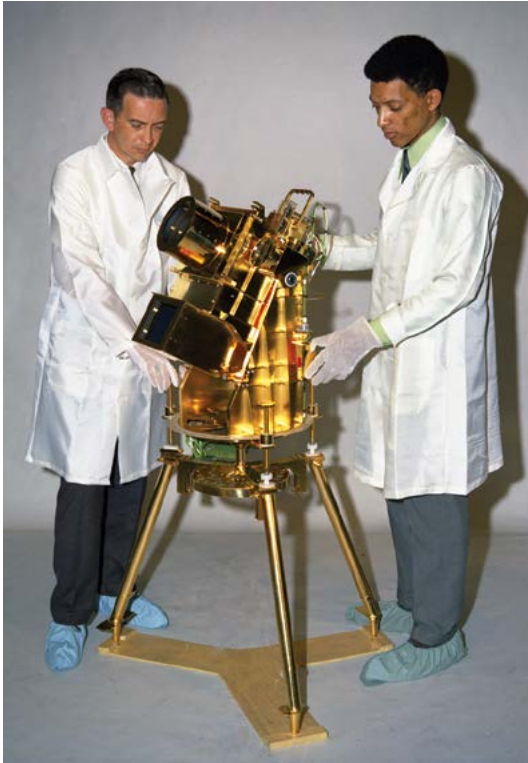
The first observatory ever operated by man from a fixed platform outside the earth was this gold-plated ultra-violet camera/spectrograph. It was placed on the moon by the Apollo 16 astronauts in April 1972. George Carruthers is right and William Conway is left.
