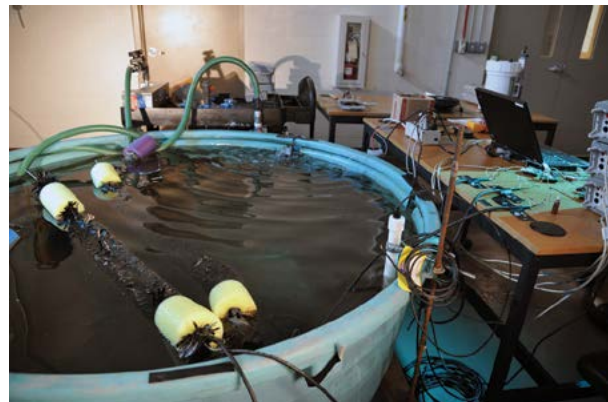
FIGURE 3 Sediment-based microbial fuel cell in the Laboratory for Autonomous Systems Research.
