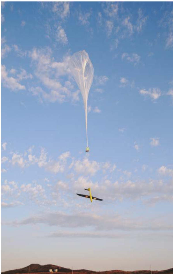
FIGURE 2 High-altitude weather balloon lifting mother-ship UAV with two CICADA vehicles attached.
