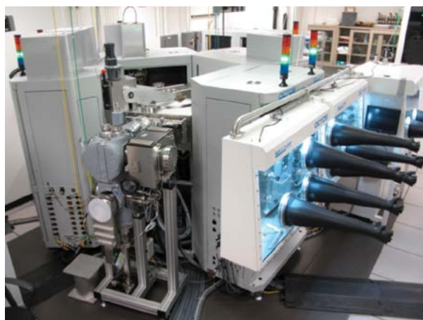
FIGURE 3 Vacuum deposition cluster tool in the Optical Sciences Division. A glove box allows sample loading and manipulation without exposure to air, and robotic transfer moves samples among chambers to build complex, multilayer devices.
