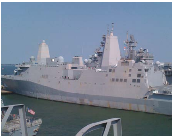
FIGURE 2 Pinking of LSA silicone alkyd coating on the USS San Antonio (LPD-17).
