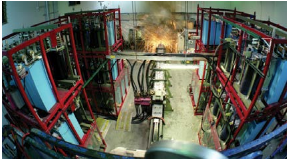
The Materials Testing Facility railgun studies the physics and material science of electromagnetic launch.
