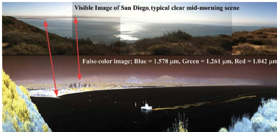
FIGURE 2 The top image is a quasi-stitched visible image of the entrance to San Diego harbor as seen from Point Loma. Below is a typical false-color image generated by the sensor using the wavelengths labeled on the image to display the hyperspectral data. The red arrows point to common locations in both representations of the scene, a breakwater on the left and downtown San Diego on the right.
