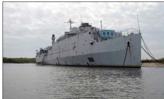
Moored in Mobile Bay, Alabama, the ex-USS Shadwell is regularly set ablaze in a controlled environment to further the safety of operational Navy and civilian firefighting measures.
