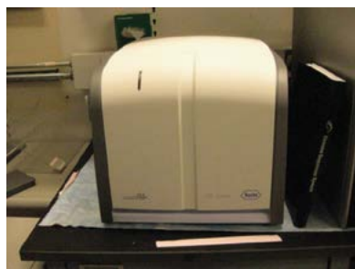
DNA Sequencer: High-throughput sequencer providing over >35 million bases per run with sequence reads averaging 450 bases in length.
