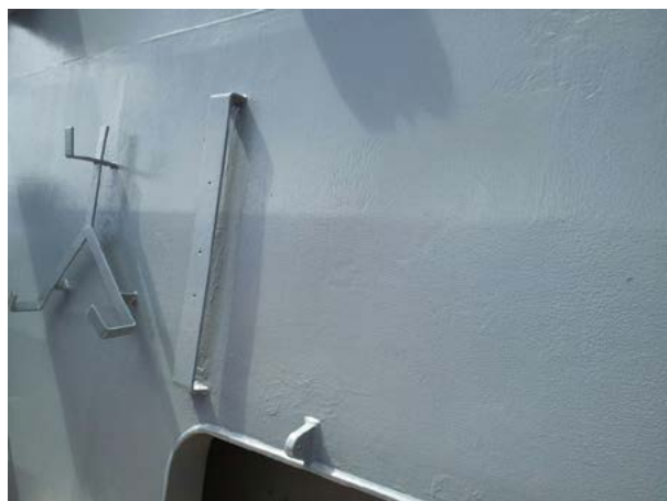
FIGURE 6 Haze Gray version of NRL's 1K polysiloxane topside coating aboard the USS Hopper (DDG-70).
