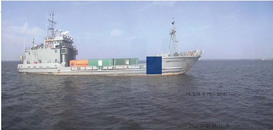
Photograph of an LCU-2000 target ship with a hidden radiation source as seen by the SuperMISTI system. The reconstructed radiation source position is overlaid as the dark blue rectangle.
