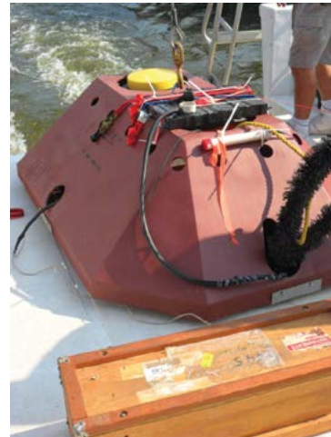
Seabed energy harvesting devices to power underwater Navy sensors.
