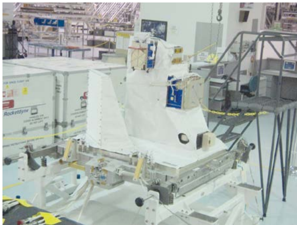
FIGURE 8 The GLADIS payload attached to STP-H4 in launch configuration.
