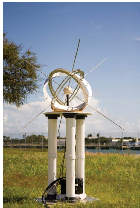
FIGURE 3 Fielded EMVS setup on 5 ft tall stand with battery to power antenna "active balun" on ground plane at base.
