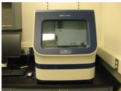
Genetic Analyzer: The Genetic Analyzer allows for presequencing sample screening and low cost fragment analysis by Length Heterogeneity-Polymerase Chain Reaction.
