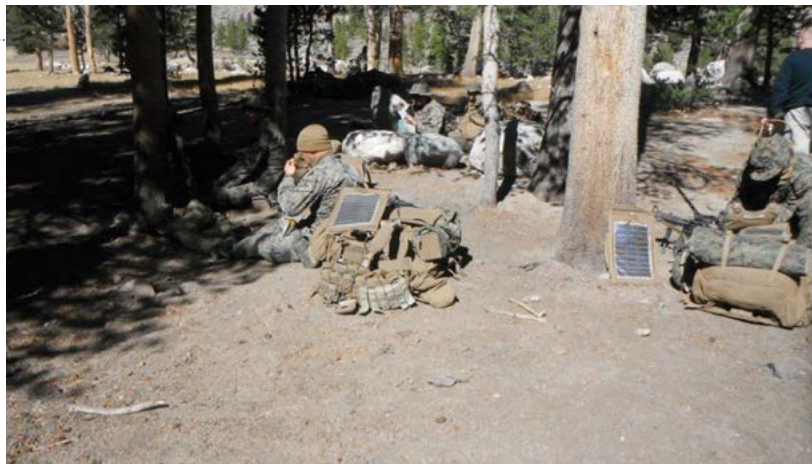
The high-efficiency, flexible solar panels developed by NRL have been integrated into the U.S. Marine Corps Marine Austere Patrolling System (MAPS), which was field-tested by Marines at the Bridgeport Mountain Training Area. Pictured here are two Marines in camp during the MAPS exercise with the solar arrays deployed. During this exercise, the solar panels were able to keep the batteries of a rifle squad, 13 Marines, charged during the entire 4-day mission, thereby eliminating the need to pack replacement batteries or for resupply.
