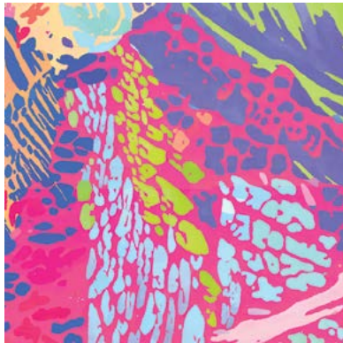
Electron backscatter diffraction inverse pole figure map shows the grain orientations of the ferrite and austenite phases in a duplex stainless steel 2205 alloy.
