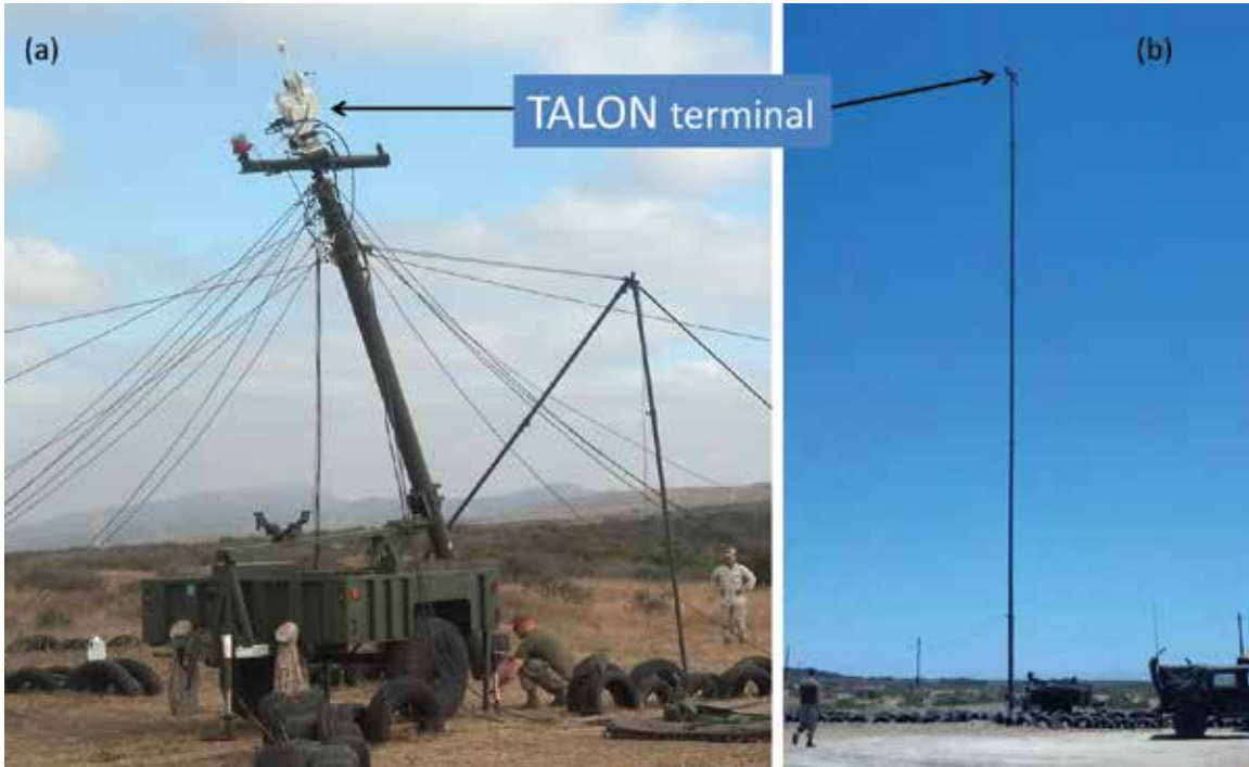
FIGURE 3 TALON terminal being raised on USMC mast (a) and mounted on mast at 100 ft elevation (b).
