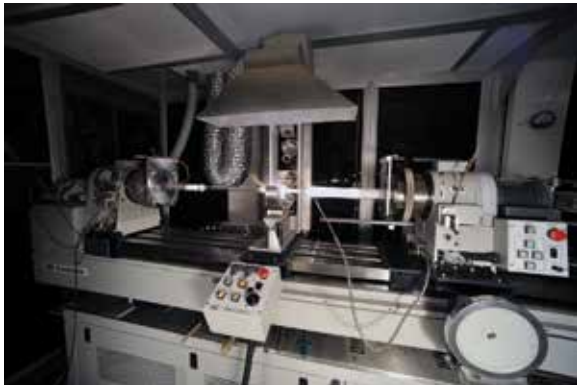
The Optical Fiber Preform Fabrication Facility includes computer control of the glass composition and standard fiber-optic dopants as well as rare earths, aluminum, and other components for specialty fibers.
