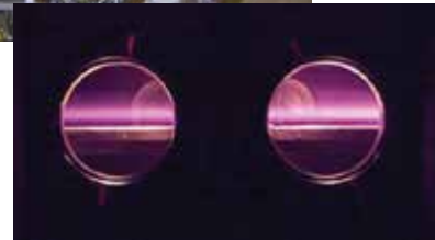
The Large Area Plasma Processing System (LAPPS) is used to develop, characterize, and study plasma-based processing of energy sensitive materials.
