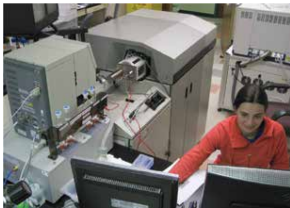
Applied Biosystems QSTAR Elite mass spectrometer coupled with a Tempo Nano Multi-Dimensional Liquid Chromatography (MDLC) System.
