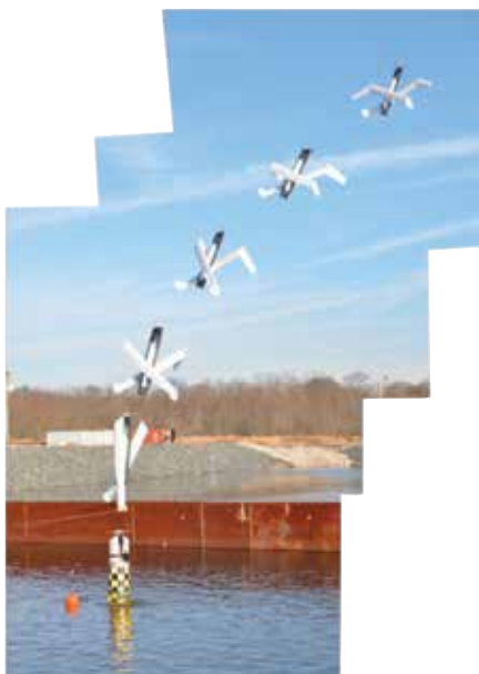
XFC (Experimental Fuel Cell) UAV — tube launch sequence.
