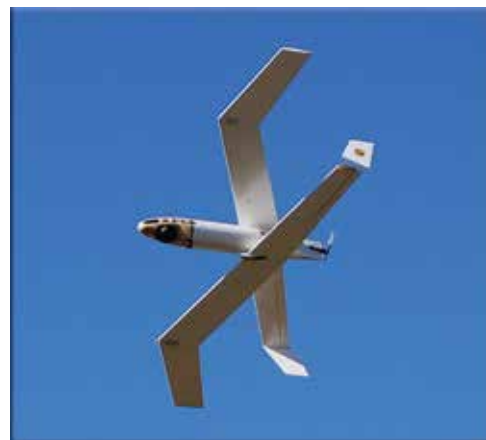
XFC prototype in flight under fuel cell power.
