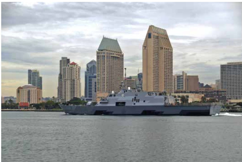
FIGURE 4 USS Fort Worth (LCS 3) exhibits NRL's camouflage paint scheme.
