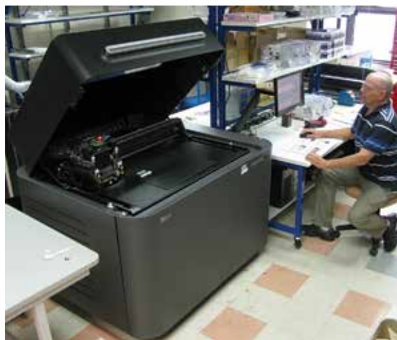
Prototyping facility 3D printer for rapid production of scale models or custom parts.
