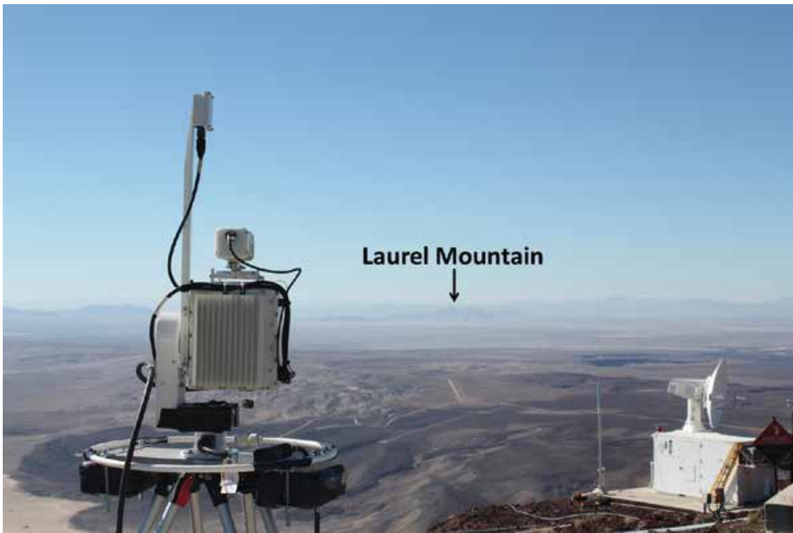
FIGURE 4 TALON terminal mounted on Cinder Peak at NAWS China Lake pointed at Laurel Mountain 50 km away.
