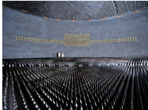
The Central Target Simulation Facility is a high-performance, hardware-in-the-loop simulator for real-time closed-loop testing and evaluation of electronic warfare systems and techniques to counter the antiship missile threats.
