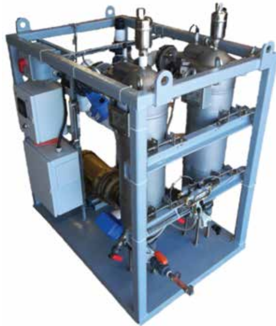
FIGURE 1 Photograph of the shipboard filter skid (the filter housings, each containing a 35 \mu\text{m} filter bag, are the silver, oblong canisters).
