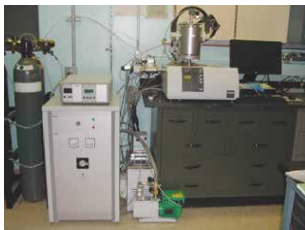
Thermal gravimetric analysis: The new simultaneous thermal analyzer NETZSCH STA 449 F3 Jupiter allows the measurement of mass changes and thermal effects (TG, TG-DTA, and TG-DSC measurements) between -150 °C and 2400 °C.
