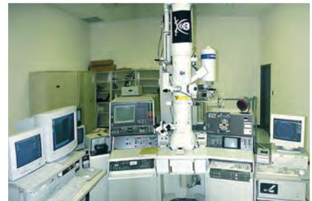
The JEOL JEM-3010 transmission electron microscope.
