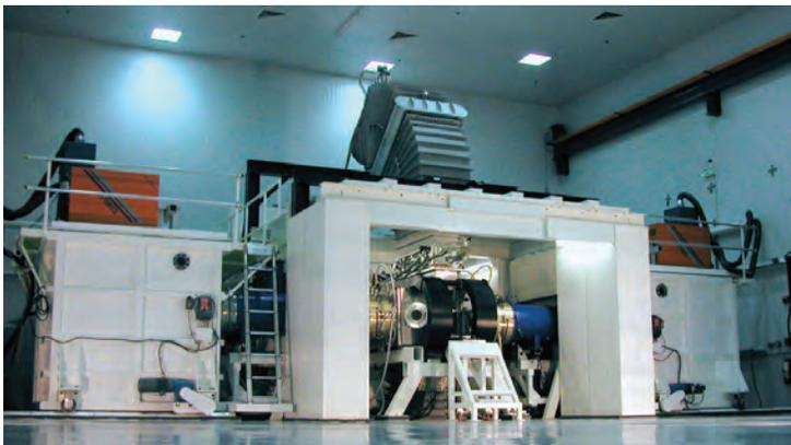
Electra repetitive electron beam facility, used to investigate inertial fusion energy, materials modification, waste remediation, and biofuel production.
