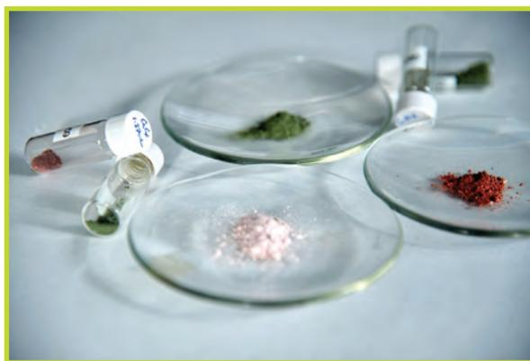
The porphyrin-functionalized organosilicate sorbents Dr. Brandy White designed at NRL capture and break down toxic industrial chemicals and other targets into things that are harmless.
