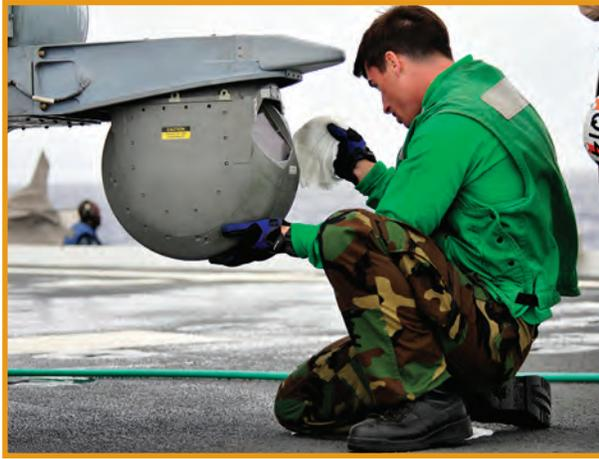
A technician cleans an infrared camera from the deck of USS *Cleveland* (LPD 7). NRL is making transparent ceramics, called spinel, that could one day replace the glass in military imaging systems.
