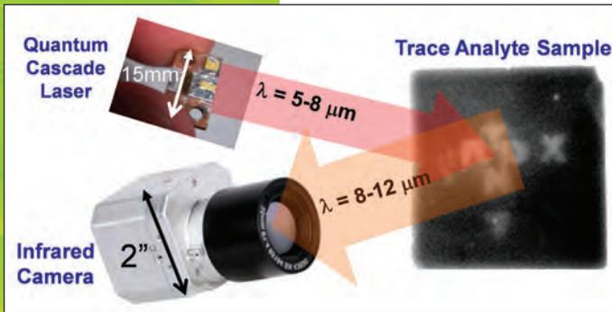
In the photothermal infrared imaging spectroscopy (PT-IRIS) technique, an infrared quantum cascade laser (QCL) is tuned through a series of wavelengths in the 5 to 8  $\mu\text{m}$  range.
