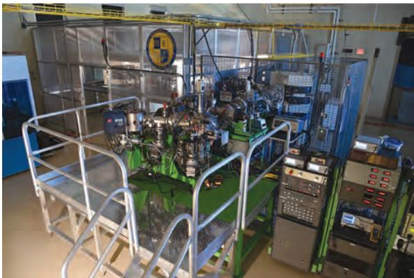
NRL-MSTD's Accelerator Mass Spectrometry Facility provides positive ion analysis of materials for trace chemical and isotope composition.
