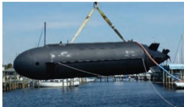
Proteus LDUUV (large displacement unmanned underwater vehicle) being launched. The Acoustics Division is developing technology for this Columbia Group vehicle and recently completed measurements with it.
