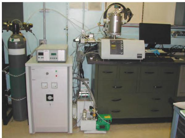
Thermal gravimetric analysis: The new simultaneous thermal analyzer NETZSCH STA 449 F3 Jupiter allows the measurement of mass changes and thermal effects (TG, TG-DTA, and TG-DSC measurements) between  $-150\text{ }^{\circ}\text{C}$  and  $2400\text{ }^{\circ}\text{C}$ .
