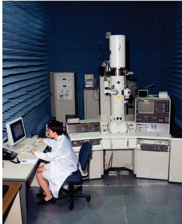
Transmission electron microscopy.
