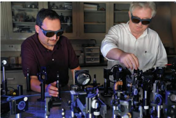
Scientists work on the alignment of an experiment designed to quantify material response to ultrashort laser pulses.
