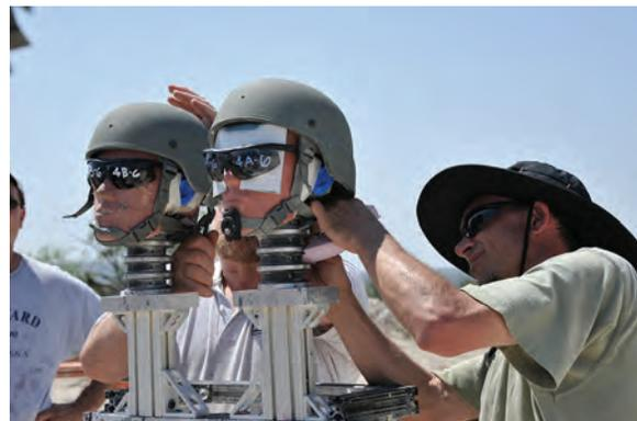
U.S. Naval Research Laboratory scientists adjust helmet and pressure sensors on Hybrid III dummies during experimental blast testing.
