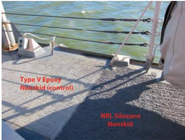
NRL's patented polysiloxane direct-to-metal nonskid coating has improved durability, color retention, and reduced VOC.
