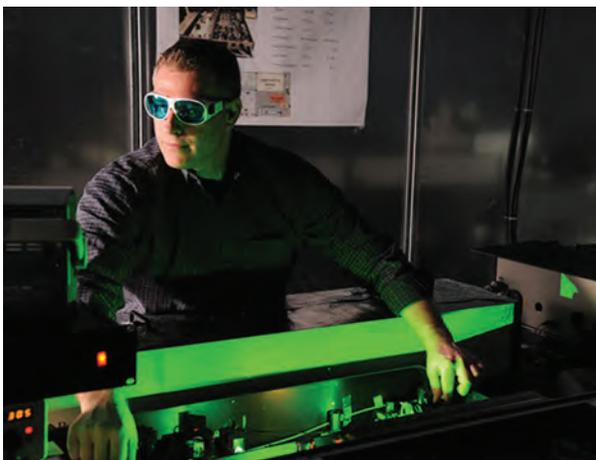
NRL research physicist aligning the TEWD 30 TW Ti:Sapphire laser system.
