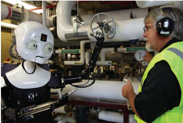
Octavia, one of three anthropomorphic robots at the Navy Center for Applied Research in Artificial Intelligence, uses and understands gestures in order to communicate in high noise environments.
