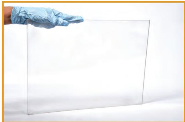
NRL uses a hot press to make spinel into conformable optics, like this flat sheet.
