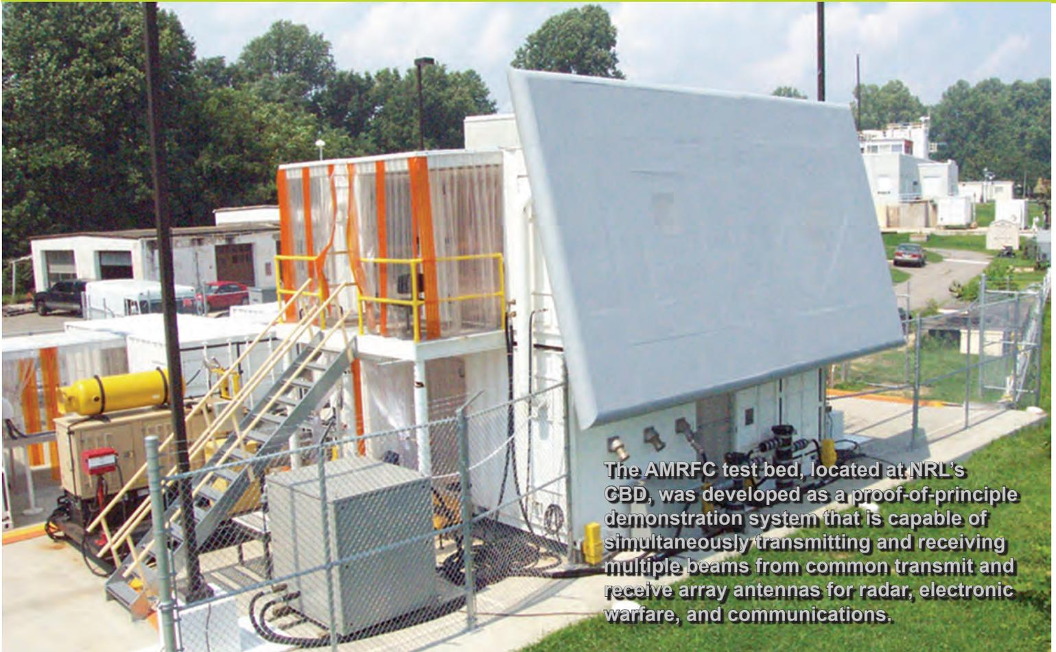
The AMRFC test bed, located at NRL's CBD, was developed as a proof-of-principle demonstration system that is capable of simultaneously transmitting and receiving multiple beams from common transmit and receive array antennas for radar, electronic warfare, and communications.
