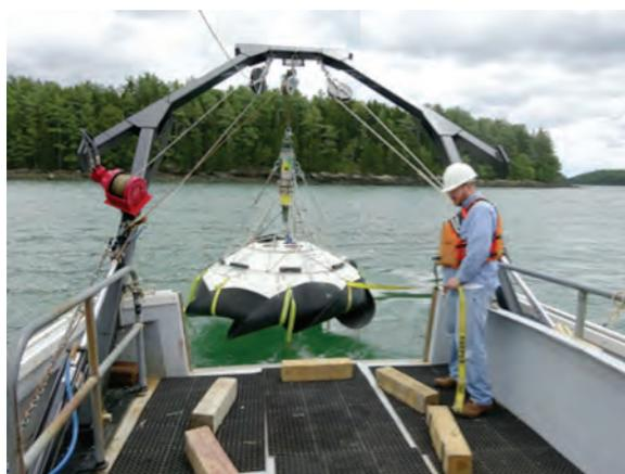
Microbe-powered ocean sensor undergoing testing in coastal Maine. Oceanographic moorings equipped with benthic microbial fuel cells (BMFCs) are being developed to persistently power oceanographic sensors. BMFCs use marine sediment organic matter as the fuel.
