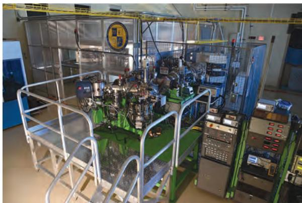
The Materials Science and Technology Division's Accelerator Mass Spectrometry Facility provides positive ion analysis of materials for trace chemical and isotope composition.
