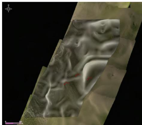
This figure shows a portion of a Nevada test range where Division researchers are studying vehicle and human trafficability. Slopes calculated from the airborne LIDAR (1 m grid) are overlaid on the airborne photogrammetry.
