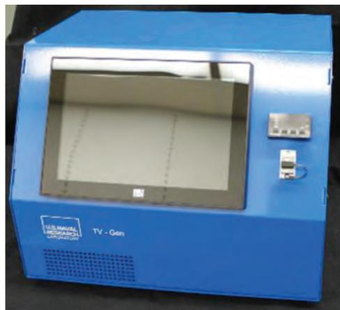
The Trace Vapor Generator for Explosives and Narcotics (TV-Gen) is a portable, compact vapor generation system capable of reproducibly and accurately generating trace vapors (parts per quadrillion to parts per million) of troublesome, low vapor pressure compounds such as explosives and narcotics for delivery to sensors and materials undergoing testing or calibration.
