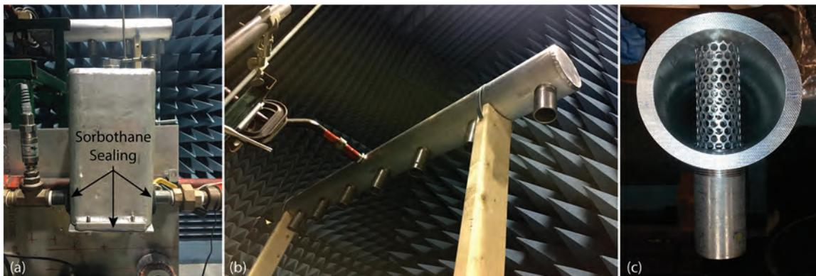
**FIGURE 3** Detail on mitigation approaches: (a) valve enclosure, (b) prototype manifold with expansion volume, and (c) perforated sheets in prototype manifold (prior to welding end) and multiple exit nozzles.
