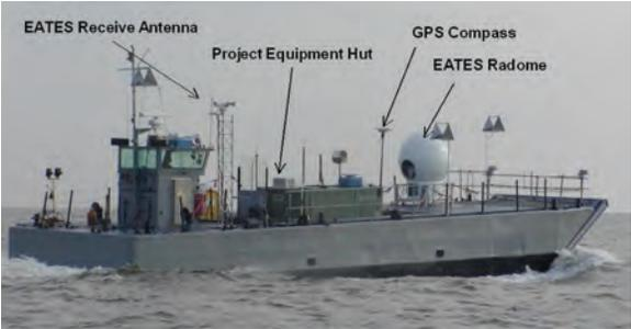
EATES — Electronic Attack Technique Evaluation System, a stand-alone portable electronic attack testing system.
