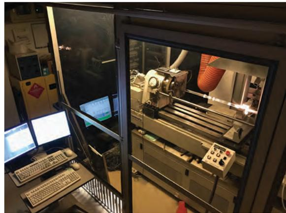
The optical sciences advanced materials group maintains unique glass processing capability. The MCVD Lathe (shown here) allows scientists to create Silica fiber preforms in which the chemical composition of the glass is tailored to achieve specific optical properties. Applications include high-power fiber lasers operating in eye safer regimes and optical fibers operating in radiation-rich environments.
