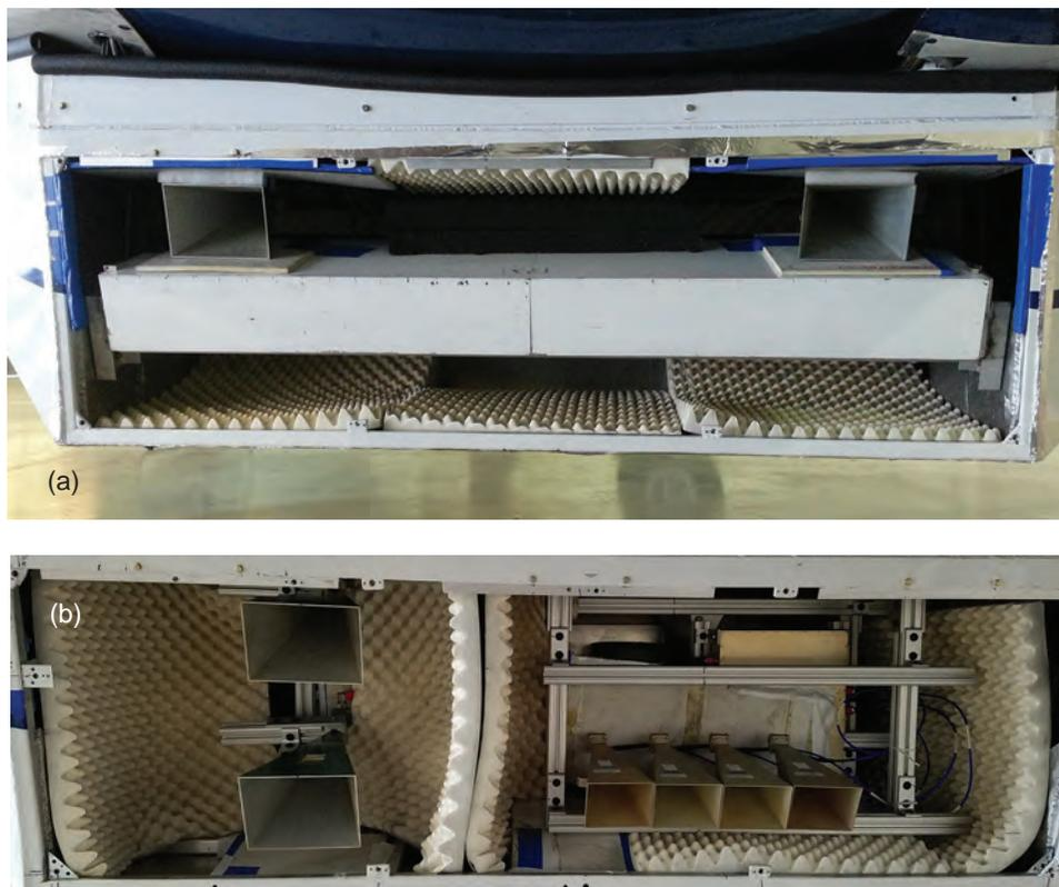
**FIGURE 7** Radome interior of the U.S. Naval Research Laboratory multichannel synthetic aperture radar (MSAR) with antennas in the (a) 32 phase center (PHC) along-track configuration, and (b) 8 PHC combined along-track/cross-track configuration.
