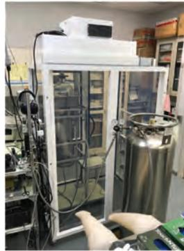
The bio-aerosol containment chamber allows NRL scientists to test the limits of new optical detection strategies aimed at providing warning in the event of a chemical or biological attack.
