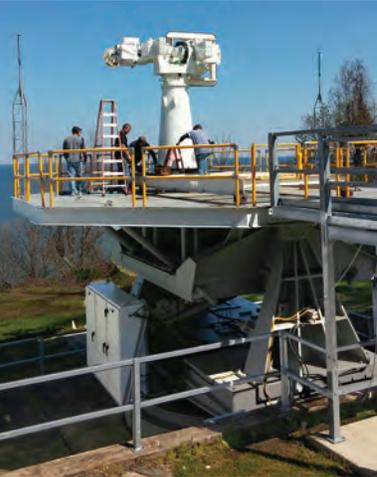
TEWD engineers prepare for dynamic testing of the 4000 lb Roll-Pitch Stabilized Antenna System mounted on NRL's Ship Motion Simulator located at the Chesapeake Bay Detachment facility.
