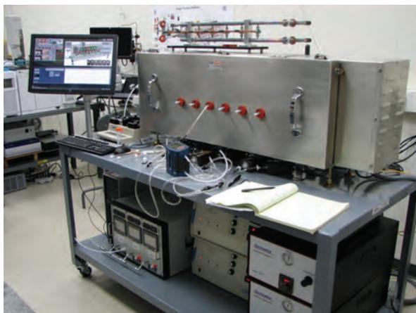
The Trace Explosives Sensor Testbed (TESTbed) has dedicated computer control of a standardized vapor delivery system with an automated data collection system suitable for obtaining high-quality data for sensor validation.
