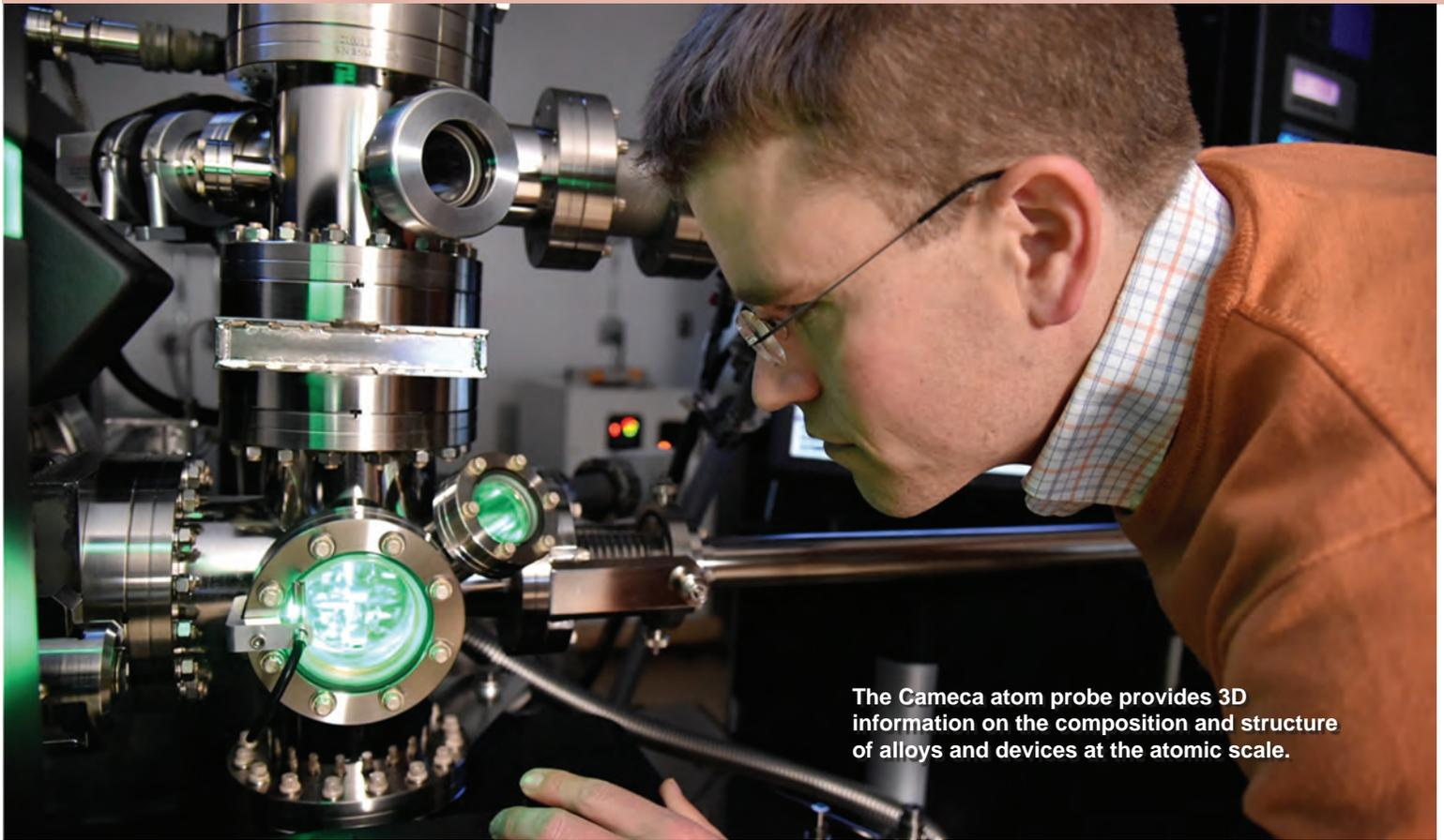
The Cameca atom probe provides 3D information on the composition and structure of alloys and devices at the atomic scale.
