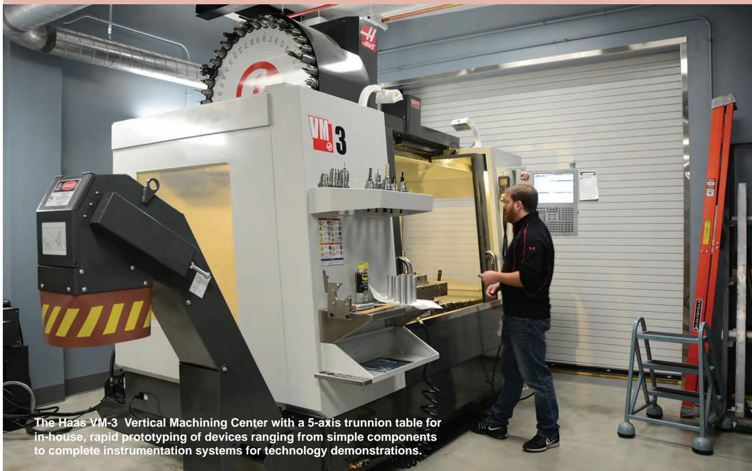
The Haas VM-3 Vertical Machining Center with a 5-axis trunnion table for in-house, rapid prototyping of devices ranging from simple components to complete instrumentation systems for technology demonstrations.
