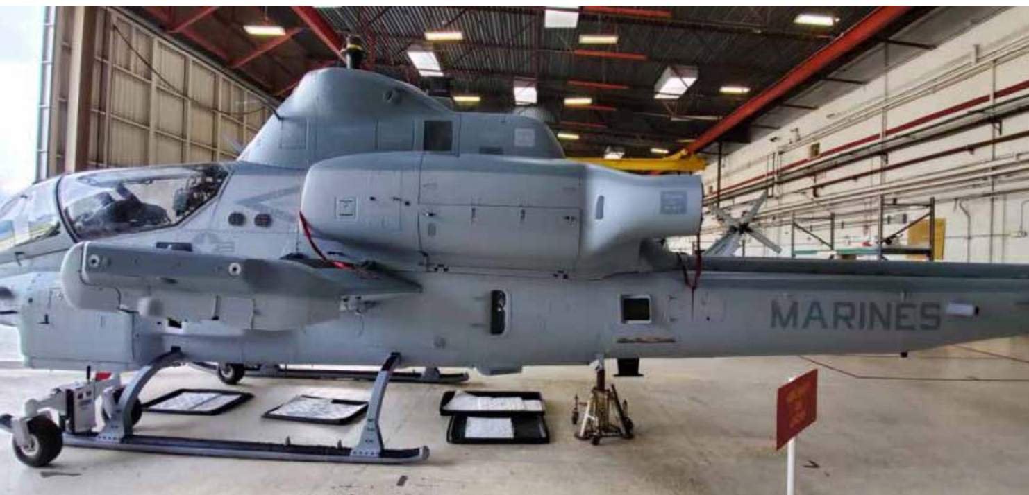
Marine Corps AH-1Z Viper helicopter is painted with one-component (1K) camouflage gray polysiloxane topcoat on the exterior. U.S. Naval Research Laboratory chemists developed the new topcoat for DoD aircraft, which is safer for the environment and easier to apply. (U.S. Naval Research Laboratory)
