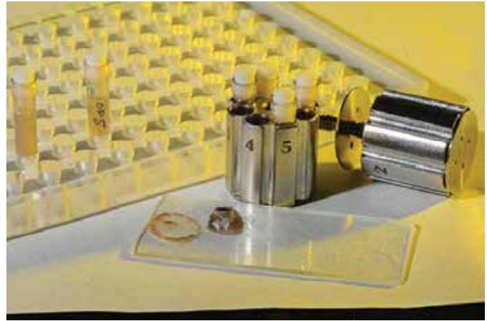
Barnacle samples in pressure cycling technology (PCT) tubes and bullet with barnacle samples in the background are used for proteomics analysis. The barnacle base plate covers the glue, illustrating how difficult sample collection is; the tubes and bullet are specially designed to handle high pressure conditions.
