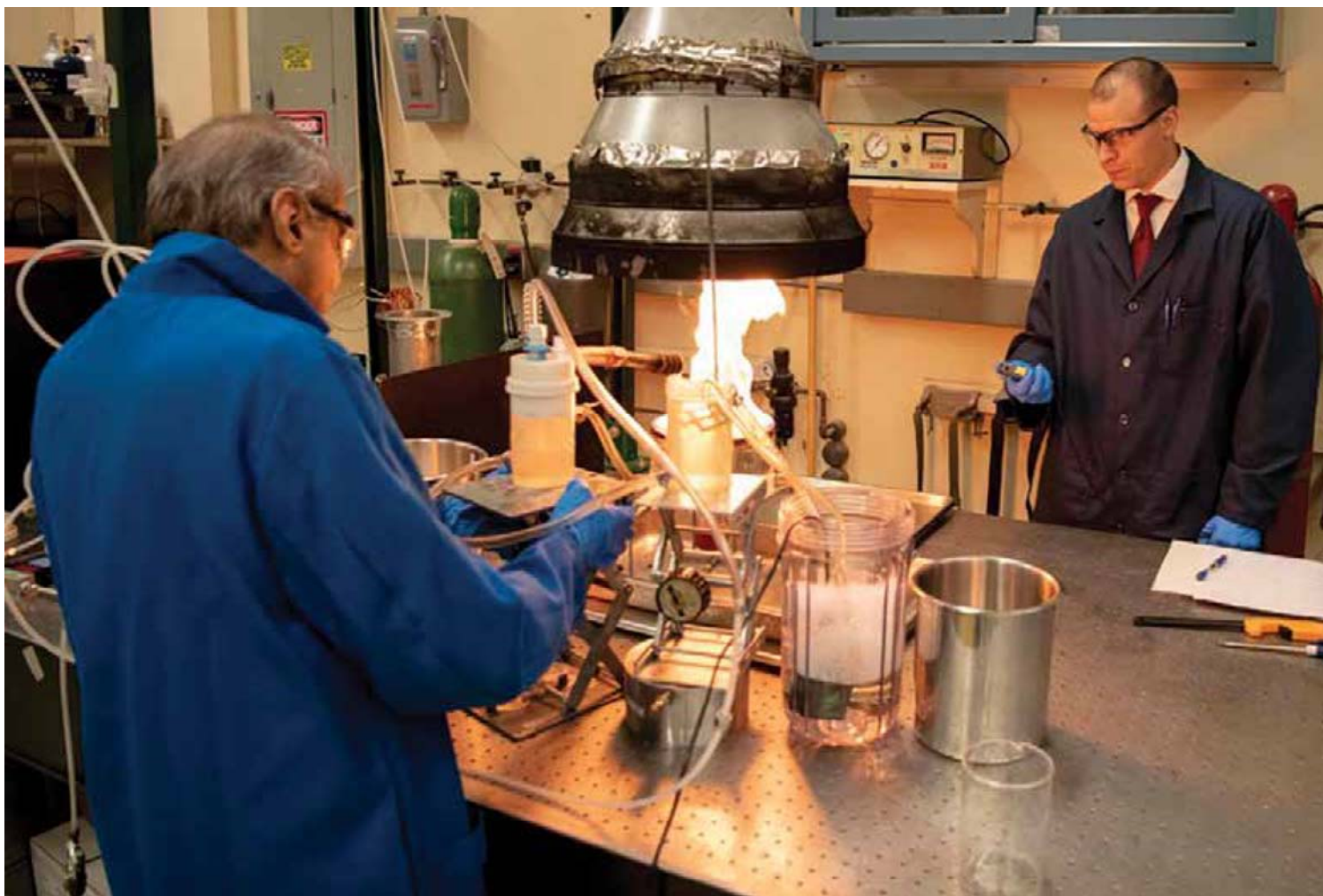
Naval Research Lab Chemical Engineer Gopal Ananth and Research Chemist Spencer Giles test an experimental aqueous film-forming foam at the NRL in Washington, Sept. 23, 2019. NRL scientists are conducting research to support the Defense Department's effort to replace firefighting foams containing fluorine.
