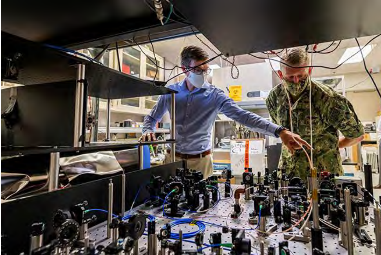
Jonathan Kwolek, Ph.D., left, a U.S. Naval Research Laboratory research physicist, shows an atom interferometer to Chief of Naval Research Rear Adm. Lorin Selby on Sept. 14, 2020, at NRL facilities in Washington, D.C. Kwolek uses the instrument to measure motion for navigational purposes. (U.S. Navy photo by Jonathan Steffen)
