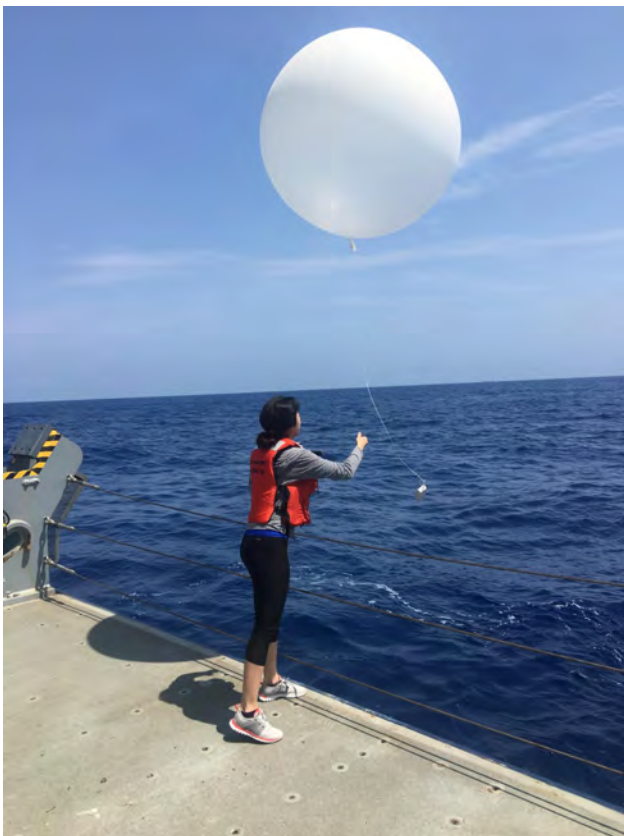
A radiosonde is deployed to record temperature, humidity, and pressure during the oceanographic cruise aboard R/V Sally Ride in the Bay of Bengal. (U.S. Navy Photo/Released)
