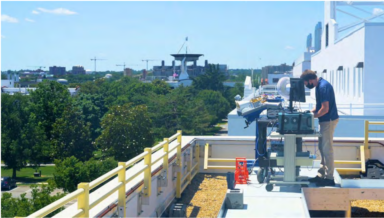
John Jakabosky, an electronics engineer from the U.S. Naval Research Laboratory's Radar Division, tests a millimeter-wave radar in Washington, D.C. The division developed a way to sense a target's subtle vibrations and to characterize the data in order to “hear” the target's activities. (U.S. Navy photo by Leonard Pieton)
