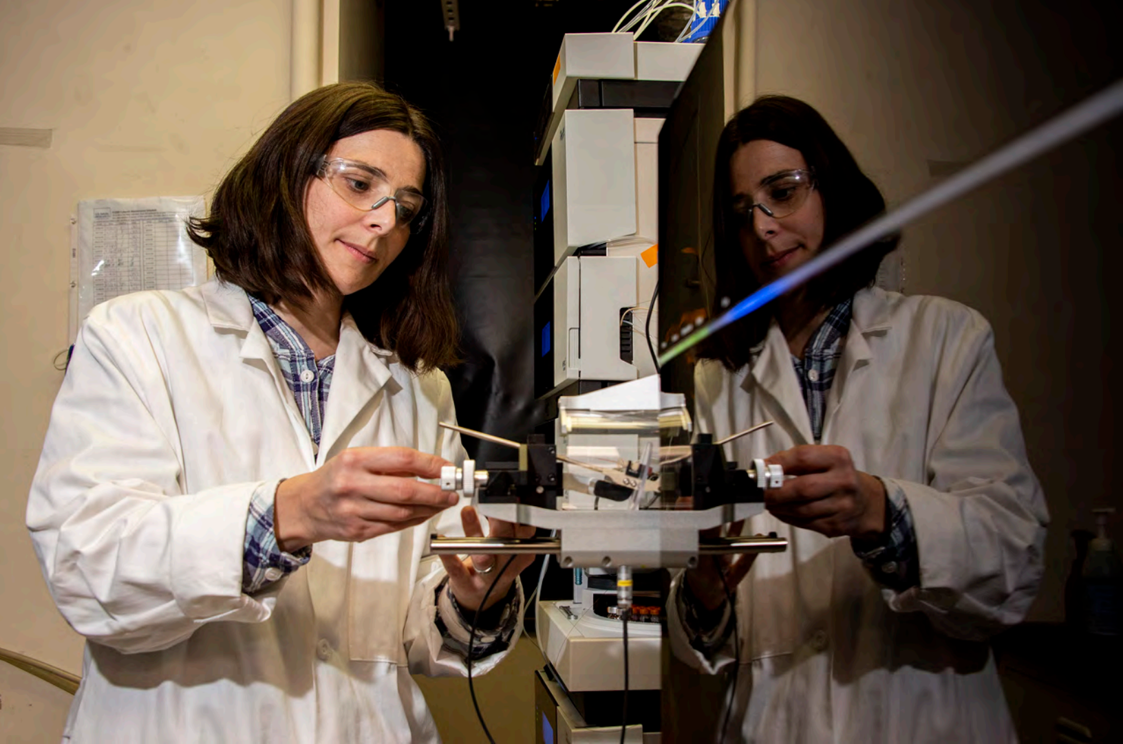
Dasha Leary, U.S. Naval Research Laboratory research biologist, prepares a liquid chromatography-mass spectrometry (LC-MS) instrument for sample analysis in Washington, D.C., on Jan. 16, 2020. This equipment allows Leary to identify protein extracts from marine microbial organisms. (U.S. Navy photo by Sarah Peterson)
