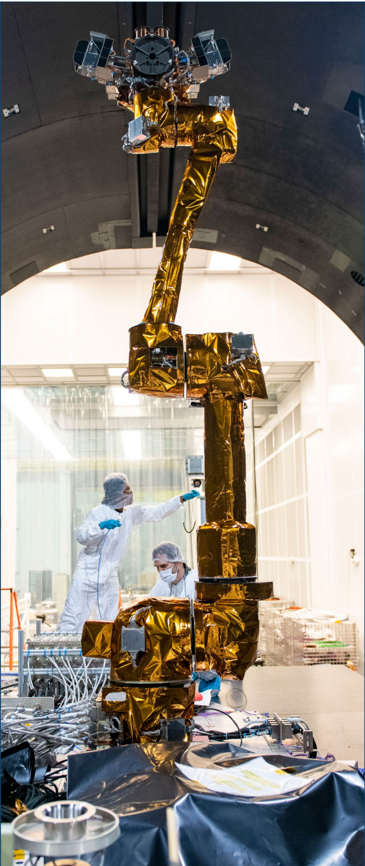
Members of the U.S. Naval Research Laboratory's Robotic Servicing of Geosynchronous Satellites (RSGS) team prepare the Robotic Arm System (RAS) for collision avoidance testing in the cryogenic thermal vacuum (TVAC) test room in Washington, D.C. June 16, 2022. The TVAC test room allows the team to collect data confirming the surroundings of the arm which provides its true position. (U.S. Navy photo by Sarah Peterson)
