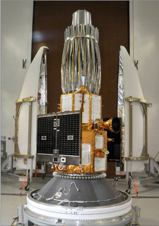
TacSat 4 was integrated with the Minotaur IV adaptor.
