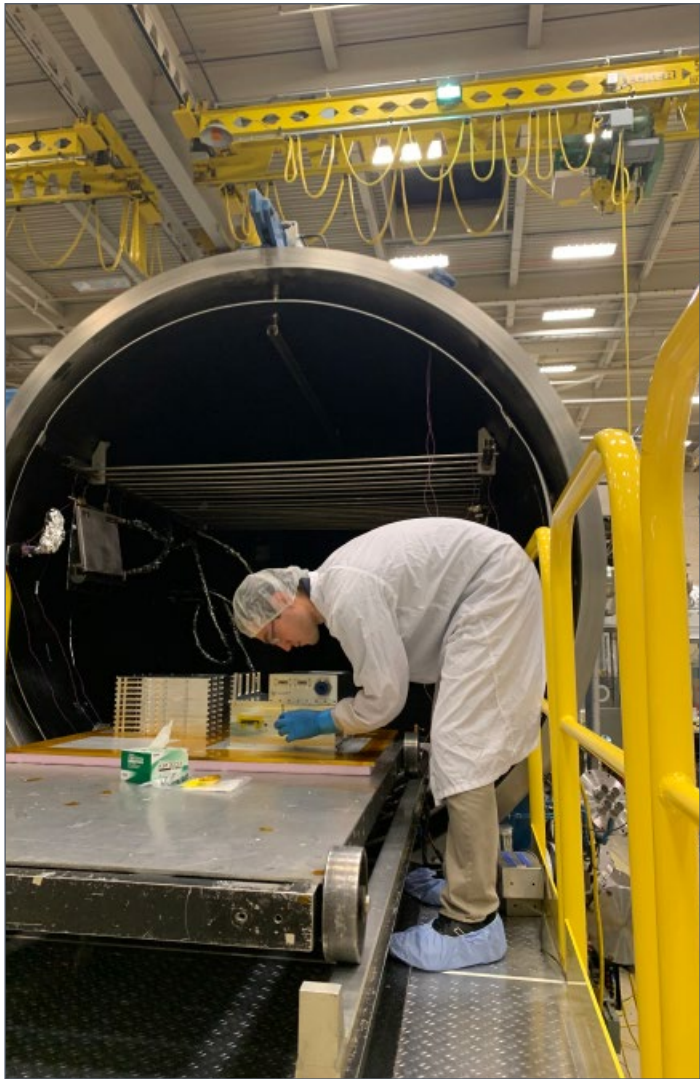
During the thermal vacuum (TVAC) test campaign at NASA’s Goddard Space Flight Center in Greenbelt, Md., in June 2023, Dr. Daniel Shy, a co-investigator on the ComPair Program, inspects the NRL-led CsI calorimeter box.
