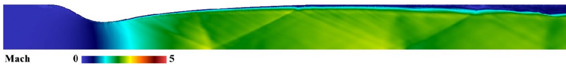
Figure 3. Mach contour of a small-scale, continuous-flow, vacuum-driven wind tunnel
