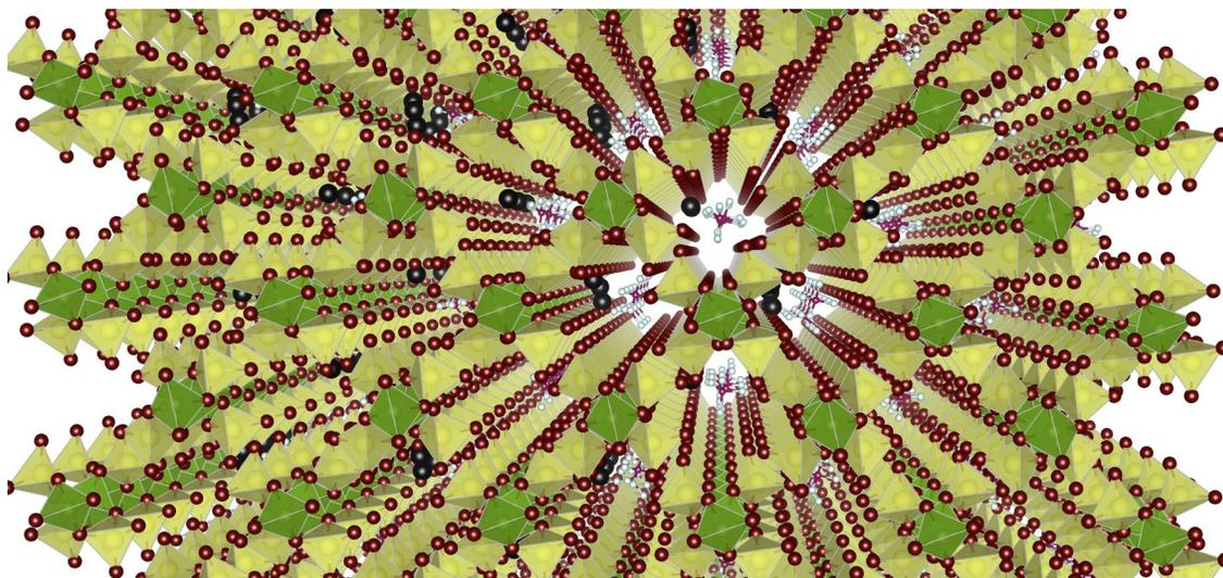
Figure 1. Relaxed structure of ammonium borosulfate ( $\text{NH}_4[\text{B}(\text{SO}_4)_2]$ ). Green polyhedra are boride units, while yellow are sulfate units. Red spheres are oxygen, light-blue spheres are hydrogen, and pink spheres are nitrogen. The black spheres represent excess protons ( $\text{p}^+$ ) at various possible positions along the three-dimensional path of conduction uncovered by density functional theory calculations.
