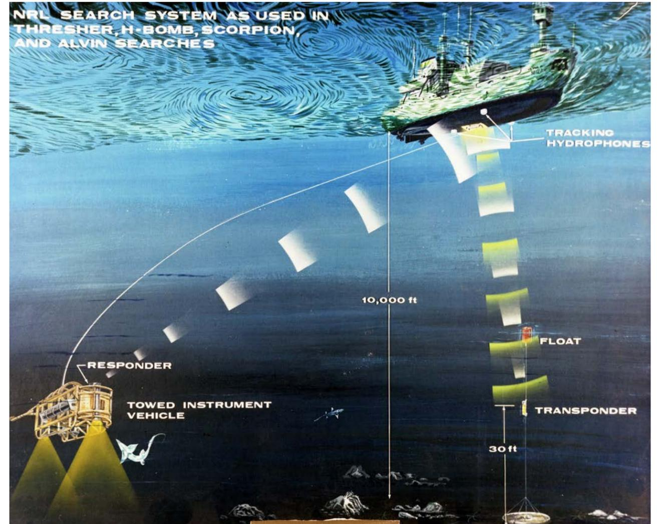
The NRL-developed Side-Looking Sonar (SILOS) sled, or "fish," was deployed aboard USS *Mizar* (T-AGOR 11) as part of several major undersea search expeditions during the 1960s, including the discovery of the lost submarines USS *Thresher* (SSN 593) and USS *Scorpion* (SSN 589). NRL graphic
