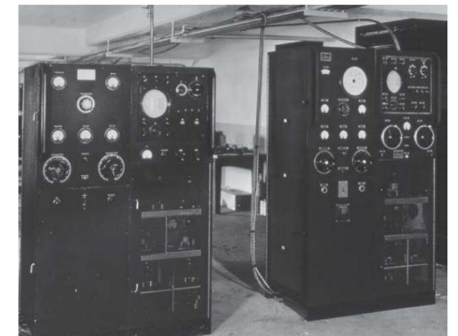
The first operational US naval radar, the CXAM-1, was the result of NRL's research efforts during the 1930s and was deployed on a variety of ship types during World War II. NRL photo
