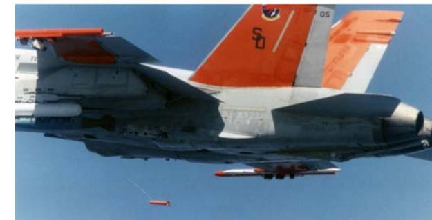
The AN/ALE-50 decoy is designed to look more like an aircraft than the aircraft itself to hostile systems. Since the 1990s, more than 25,000 decoys have been delivered for use on the F-16, F/A-18E/F, and B-1B aircraft. NRL photo
