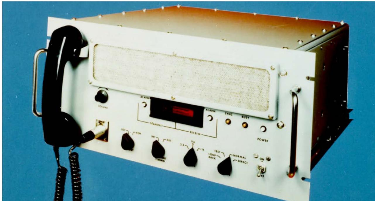
NRL developed the world's first Linear Predictive Coder in 1973, greatly improving secure voice communications. This third-generation Secure Voice Systems-2B Subscriber Terminal Unit provided office to office communication at 2400 and 4800 bits per second. NRL photo
