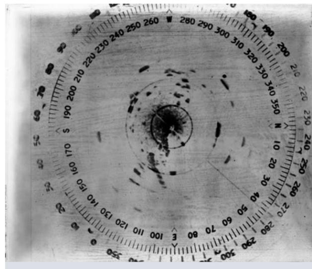
NRL originated the radar Plan-Position Indicator (PPI) in 1939. The PPI is still universally used by military and commercial organizations for the display of radar information. NRL photo
