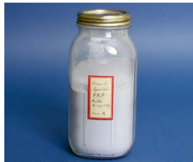
In 1959, a series of investigations by NRL in the area of chemical flame extinction gave birth to the discovery of a new dry chemical agent called potassium bicarbonate powder—or "Purple-K-powder"—used for chemical liquid fire protection. NRL photo
