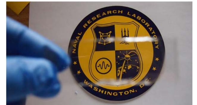
Spinel, developed at NRL during the 2000s, is a form of transparent armor made from magnesium aluminate. NRL photo
