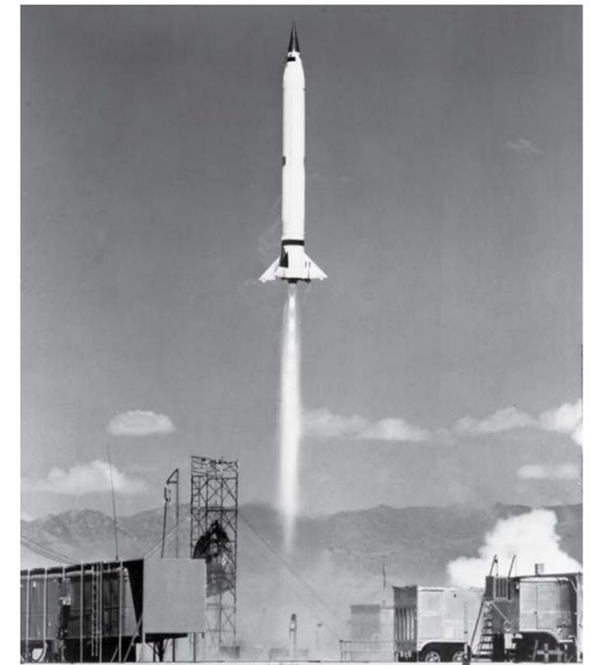
In 1946, NRL developed the Viking sounding rocket, the first rocket designed specifically for research purposes and the first to use attitude control. A total of 14 Viking rockets were launched by NRL between 1949-57. NRL photo
