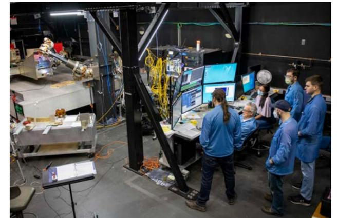
The NRL Robotic Servicing of Geosynchronous Satellites (RSGS) integration and test team analyzes data collected from contact dynamic testing on a robotic test bed in 2022. Contact dynamic testing allows the team to characterize how the payload will behave when servicing client spacecraft. Photo by Sarah Peterson, NRL
