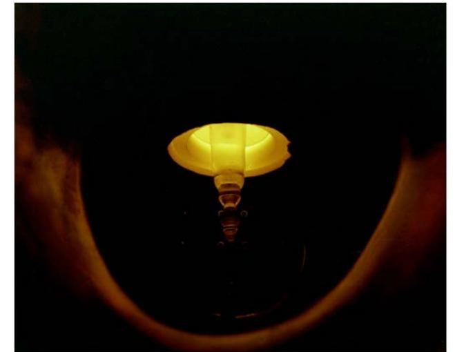
In the 1970s, NRL developed a method for compounding and growing high-purity, single crystals of gallium arsenide. Wafers made from these crystals are critical to produce high-performance microwave and millimeter-wave devices, integrated circuits, microcircuits, and transistors. NRL photo
