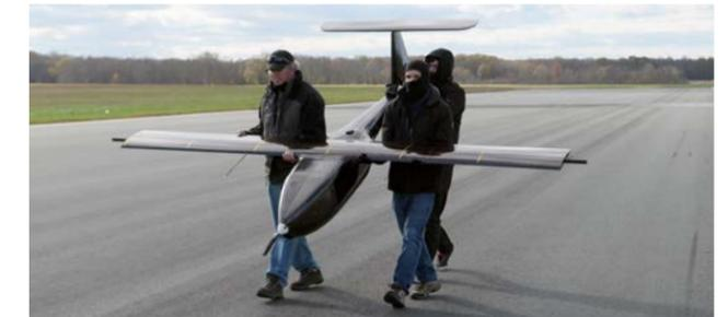
In 2011, NRL developed the Hybrid Tiger unmanned aerial vehicle, demonstrating the feasibility of using a hybrid electric-and-gas propulsion system for unmanned vehicles. NRL photo
