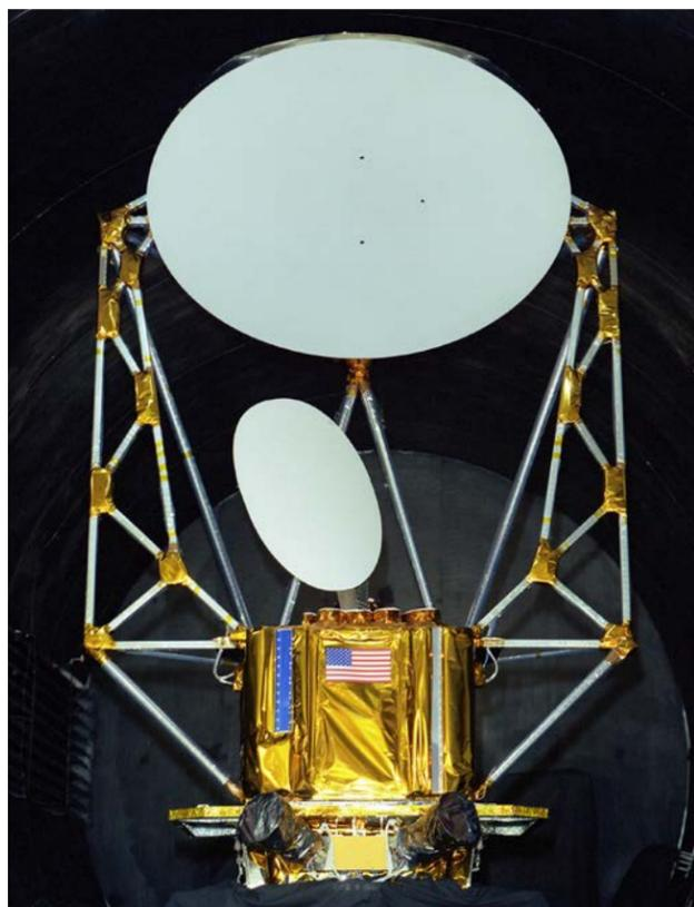
WindSat, launched in 2003, was built to retrieve the ocean wind speed and direction from space. NOAA photo
