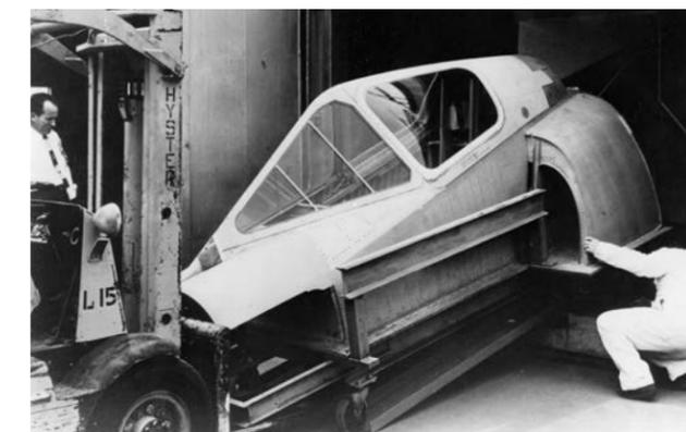
NRL researchers devised a new technique of acrylic "hot stretching" that significantly improved the toughness of aircraft canopy material, such as on this Convair F-102 Delta Dagger. The new material was stronger, lighter, and more long-lasting than anything before. NRL photo
