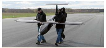
In 2011, NRL developed the Hybrid Tiger unmanned aerial vehicle, demonstrating the feasibility of using a hybrid electricand-gas propulsion system for unmanned vehicles. NRL photo
