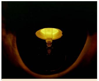
In the 1970s, NRL developed a method for compounding and growing high-purity, single crystals of gallium arsenide. Wafers made from these crystals are critical to produce high-performance microwave and millimeter-wave devices, integrated circuits, microcircuits, and transistors. NRL photo
