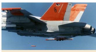
The AN/ALE-50 decoy is designed to look more like an aircraft than the aircraft itself to hostile systems. Since the 1990s, more than 25,000 decoys have been delivered for use on the F-16, F/A-18E/F, and B-1B aircraft. NRL photo
