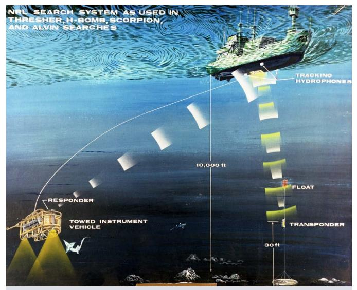
The NRL-developed Side-Looking Sonar (SILOS) sled, or "fish," was deployed aboard USS *Mizar* (T-AGOR 11) as part of several major undersea search expeditions during the 1960s, including the discovery of the lost submarines USS *Thresher* (SSN 593) and USS *Scorpion* (SSN 589). NRL graphic
