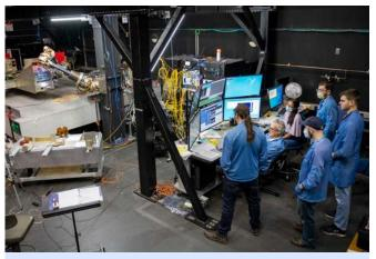
The NRL Robotic Servicing of Geosynchronous Satellites (RSGS) integration and test team analyzes data collected from contact dynamic testing on a robotic test bed in 2022. Contact dynamic testing allows the team to characterize how the payload will behave when servicing client spacecraft. Photo by Sarah Peterson, NRL
