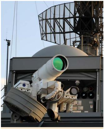
In 2014, the first operational naval laser weapon system was installed aboard USS Ponce (AFSB (I) 15) to test the viability of directed-energy weapons in an operational environment. Photo by John F. Williams
