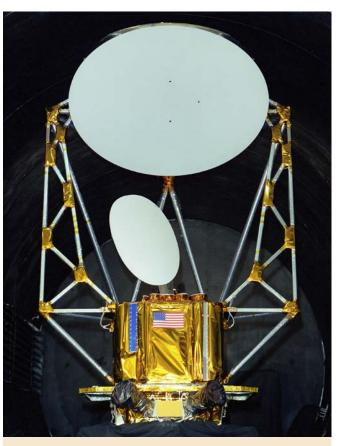
WindSat, launched in 2003, was built to retrieve the ocean wind speed and direction from space. NOAA photo
