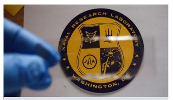
Spinel, developed at NRL during the 2000s, is a form of transparent armor made from magnesium aluminate. NRL photo
