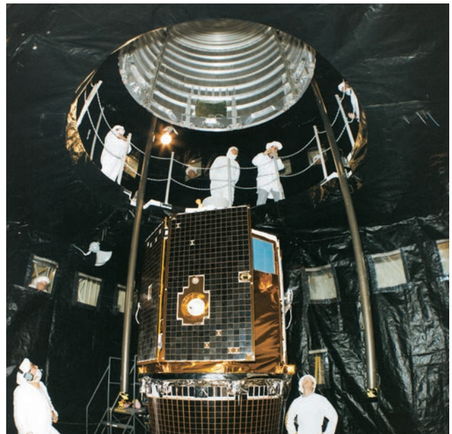
This is a final look at the Clementine DSPSE spacecraft, which is mated to its launch vehicle, the Titan IIG (two i’s, not two ones). Here, the nose fairing is being lowered to enclose Clementine in its new home during launch.
