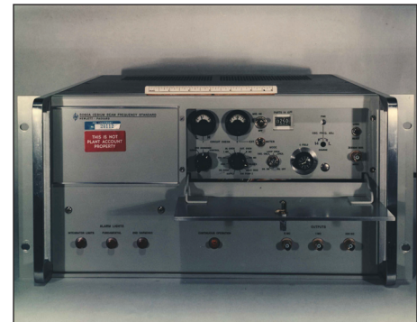
Hewlett-Packard 5060A Cesium Beam Frequency Standard. (NRL photo)
