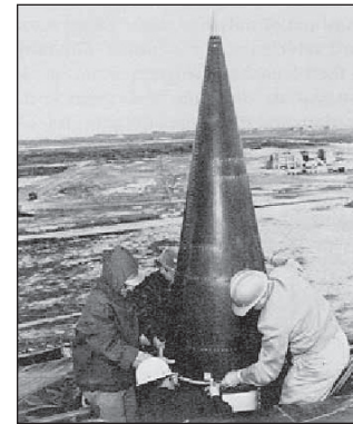
Vanguard nosecone being fitted into position prior to launch. (NASA SP-4202 2 )
