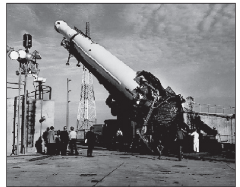
Erecting the TIMATION I launch vehicle. (NRL Photo)
