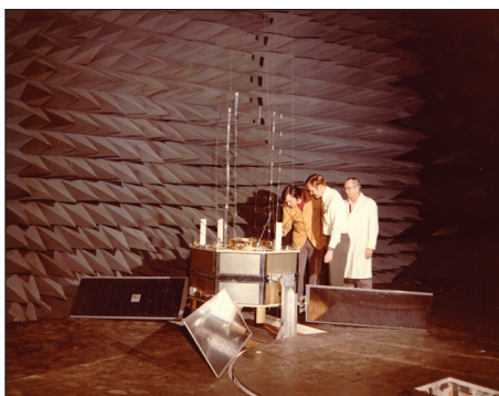
NTS-1 satellite in NRL anechoic chamber. (NRL Photo)
