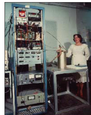
NRL Passive Space Advanced Development Model maser. (Beard-2002, p. 4. See also Beard-1986, p. 52)
