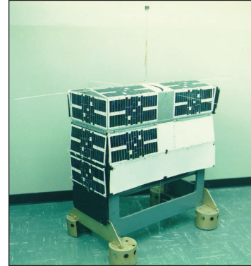
TIMATION II in the lab, with solar panels extended. (NRL Photo)
