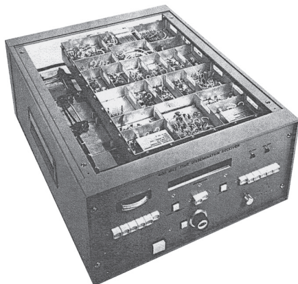
400 Megahertz time dissemination receiver. (Easton-1971, p. 59)
