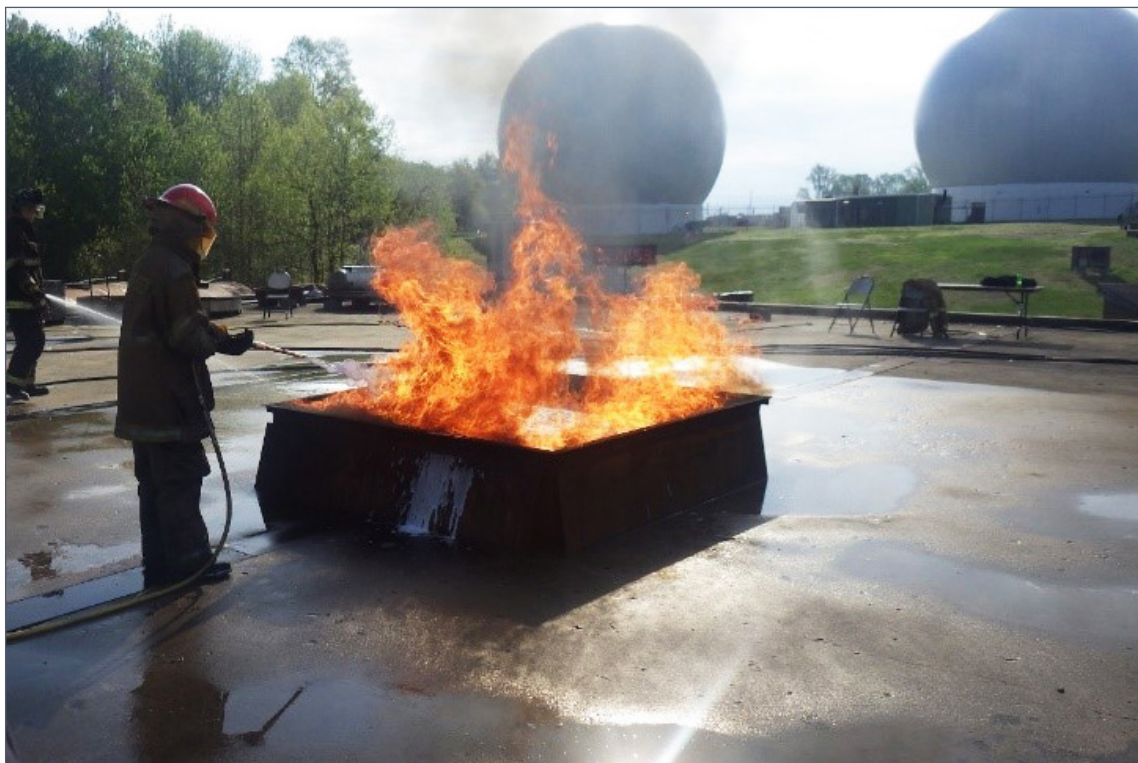
John Farley, director of fire test operations at the U.S. Naval Research Laboratory (NRL), conducts a National Fire Protection Association (NFPA) Research Foundation fluorine-free foam "Standard for Safety Foam Equipment and Liquid Concentrates" (UL-162) 50 ft 2 fire test, which was one of the 165 fire test series conducted for the NFPA at the NRL Chesapeake Bay Detachment in Chesapeake Beach, Md., in June 2019. The fire testing was conducted in calendar year 2019 and the final report, "Evaluation of the fire protection effectiveness of fluorine-free foams," was published in January 2020. (Photo courtesy Jensen Hughes Inc.)
