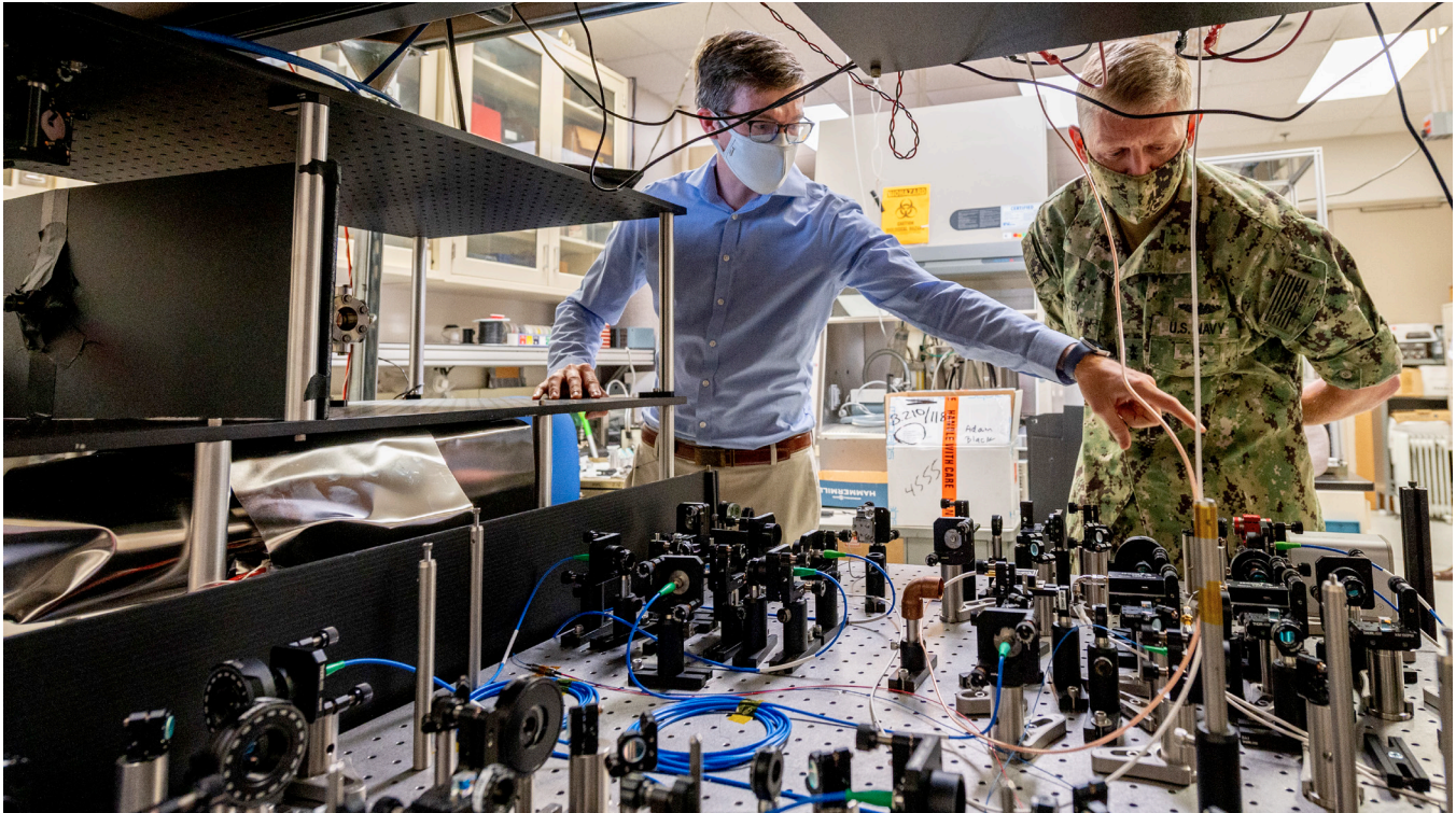
Jonathan Kwolek, a U.S. Naval Research Laboratory (NRL) research physicist, shows an atom interferometer to Chief of Naval Research Rear Adm. Lorin Selby on Sept. 14, 2020, at NRL facilities in Washington, D.C. Kwolek uses the instrument to measure motion for navigational purposes. NRL is designated as the Navy's Quantum Information Research Center. (U.S. Navy photo by Jonathan Steffen)
