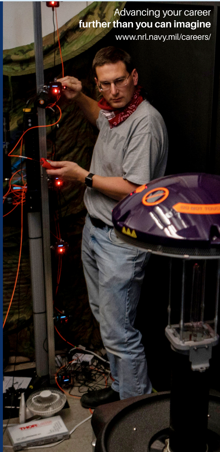
Brett Huhman, a U.S. Naval Research Laboratory senior research engineer, aligns a linear array of six photodetectors co-located with ultraviolet (UV) dosimeters and a single spectrometer during testing of a pulsed xenon gas lamp source in Washington, D.C., on May 8, 2020. Huhman was testing a variety of commercial UV light sources that might have niche applications against COVID-19 for Navy and Marine Corps environments. (U.S. Navy photo by Jonathan Steffen)
