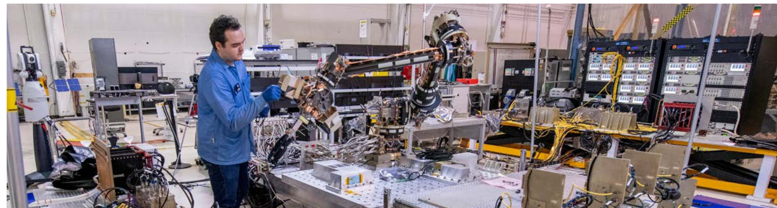
The U.S. Naval Research Laboratory's Robotic Servicing of Geosynchronous Satellites (RSGS) integration and test team analyzes data collected from contact dynamic testing on the robotic test bed in Washington, D.C., on June 16, 2022. Contact dynamic testing allows the team to characterize how the payload will behave when servicing client spacecraft. (U.S. Navy photo by Sarah Peterson)
