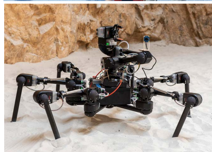
The U.S. Naval Research Laboratory's (NRL) Distributed Autonomous Systems Group demonstrates how a hexapod robot can maneuver through different terrains at NRL in Washington, D.C., on July 20, 2021. The hexapod tracks human movement in order to fulfill military communication needs. (U.S. Navy photo by Sarah Peterson)
