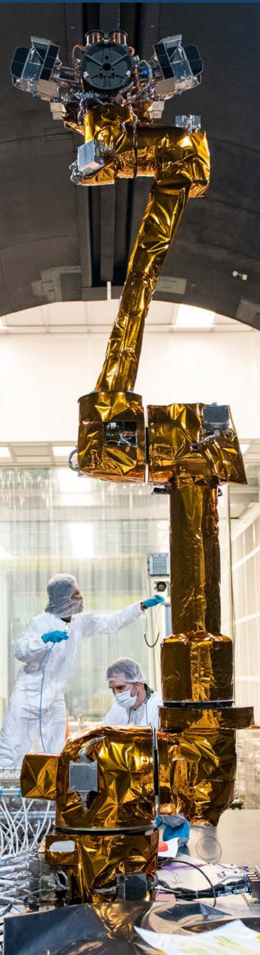
The U.S. Naval Research Laboratory's Robotic Servicing of Geosynchronous Satellites (RSGS) integration and test team analyzes data collected from contact dynamic testing on the robotic test bed in Washington, D.C., on June 16, 2022. Contact dynamic testing allows the team to characterize how the payload will behave when servicing client spacecraft. (U.S. Navy photo by Sarah Peterson)
