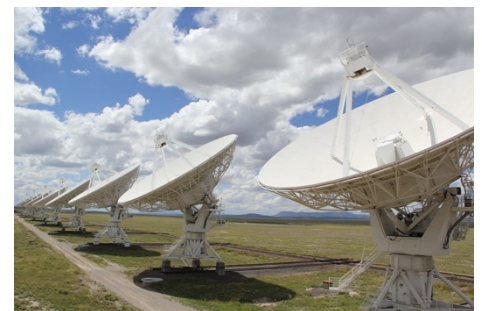
The National Radio Astronomy Observatory's Very Large Array consists of 27 antennas (25m each) operating in reconfigurable arrays from a compact 1 km array to an extended 36 km array. Photo credit: T. Clarke/NRL
