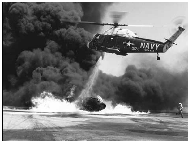
A helicopter applies NRL-developed “light water” to suppress an aircraft fire.
