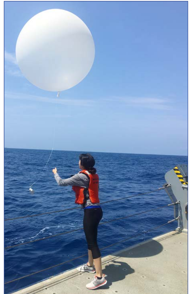
Deployment of a radiosonde to record temperature, humidity, and pressure during the oceanographic cruise aboard R/V Sally Ride in the Bay of Bengal. (U.S. Navy photo)
