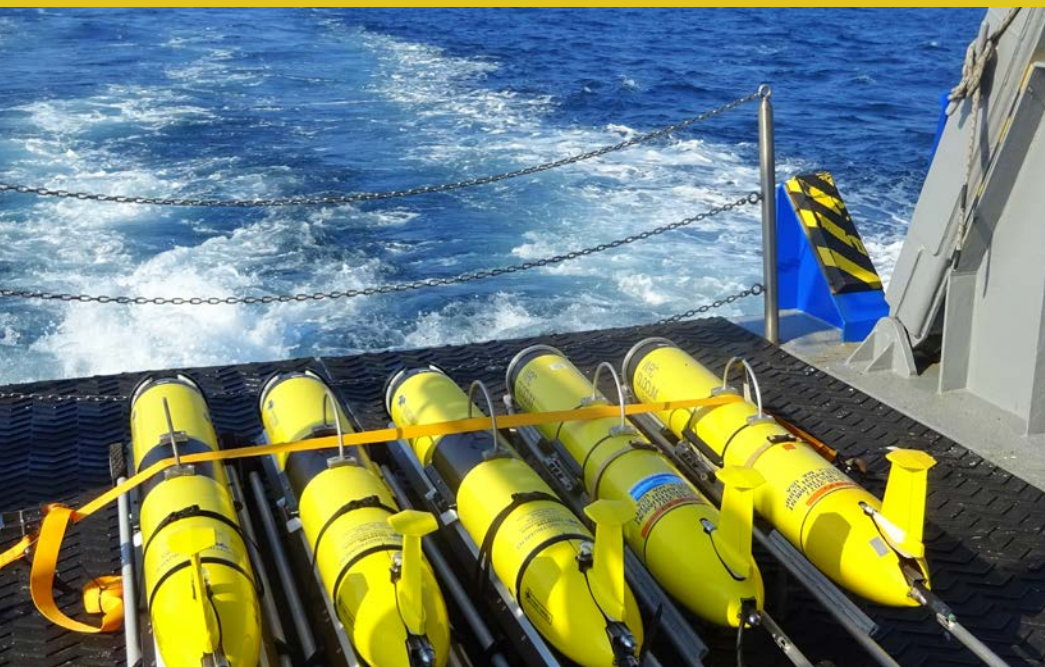
The U.S. Navy maintains a large fleet of sea gliders for environmental measurement. Sea gliders are slow-moving, long-endurance, underwater vehicles that gather data as they travel through the ocean's interior using high-efficiency buoyancy engines. (U.S. Naval Research Laboratory photo)
