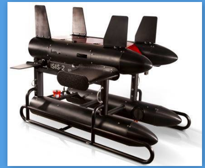
In situ ichthyoplankton imaging system (ISiIS), Remotely Operated Towed Vehicle. (Photo courtesy of Ocean Innovations)
