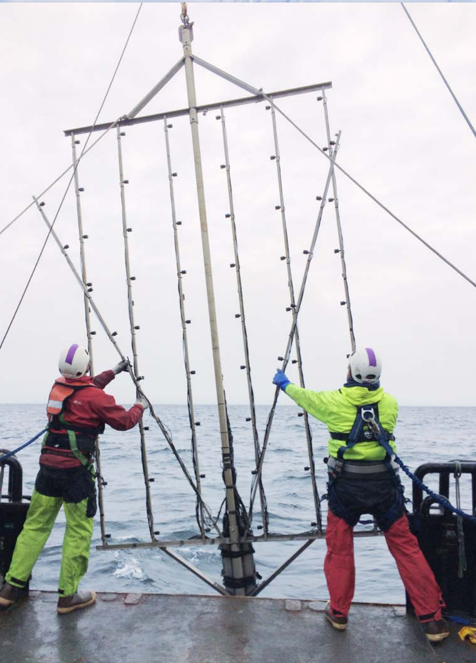
The U.S. Naval Research Laboratory-built Billboard Array is an acoustics instrument equipped with 64 receiver elements. It differentiates and amplifies sounds from different directions. The array provided remarkable acoustic data under both seasonal oceanographic and sea ice conditions during the multi-institutional Canadian Basin Acoustic Propagation Experiment (CANAPE) in the Beaufort and Chukchi seas. (U.S. Navy photo)
