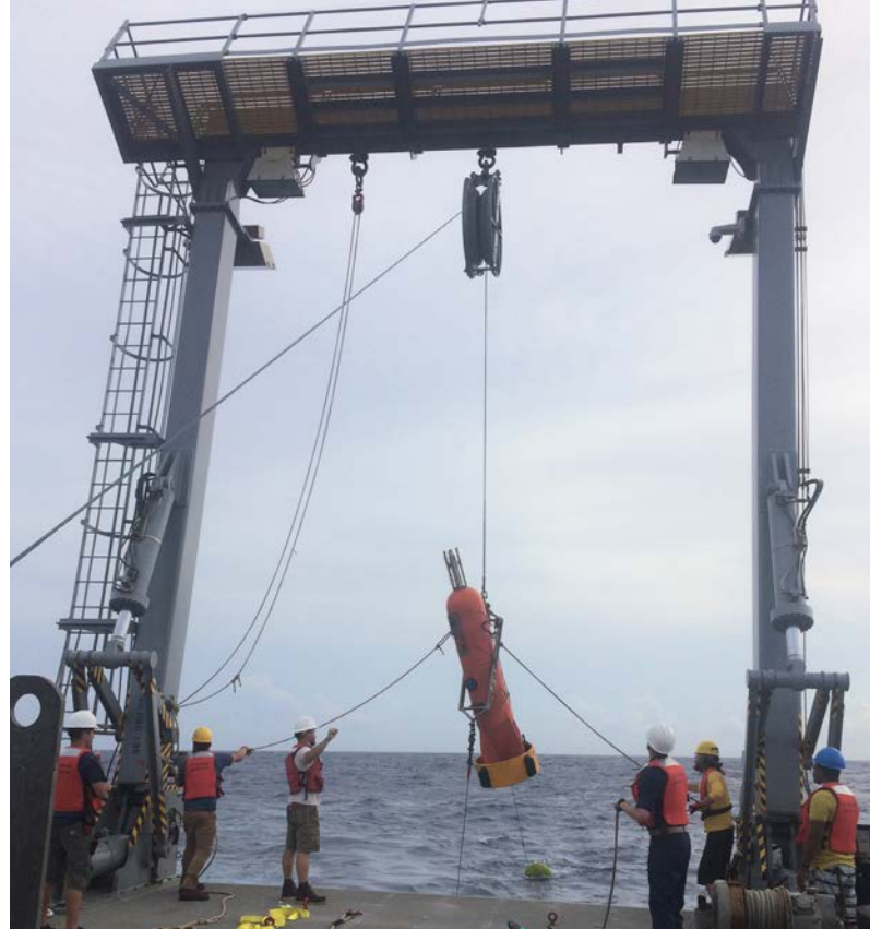
Researchers recover a large buoy housed to a velocity and temperature microstructure package during the oceanographic cruise aboard R/V Sally Ride in the Bay of Bengal. (U.S. Navy Photo)
