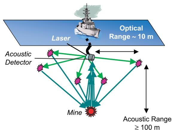
**FIGURE 5** A schematic of a laser-based acoustic imaging application shows laser light (light green) propagating to predetermined acoustic generation locations (purple), and the resulting acoustic pulses propagating to and scattering from a target (blue-green).
