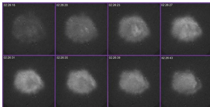
**FIGURE 3** Sequence of images of the glow plasma discharge produced with transmissions at the 3rd electron gyro harmonic using the HAARP HF transmitter in Alaska. The 3rd harmonic artificial glow plasma clouds were obtained with HAARP using transmissions at 4.34 MHz. The resonant frequency yielded green line (557.7 nm) emission with HF on 12 November 2012 between the times of 02:26:15 and 02:26:45 GMT. (Images provided by Elizabeth Kendall of SRI International)
