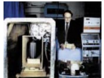
This NQR approach has been demonstrated for RDX-based explosives in a laboratory setting. The technology can be extended to detect other nitrogenous explosives as well as certain drugs of abuse. As envisioned, such an NQR explosives detector could be useful in airports and other fixed site installations.
