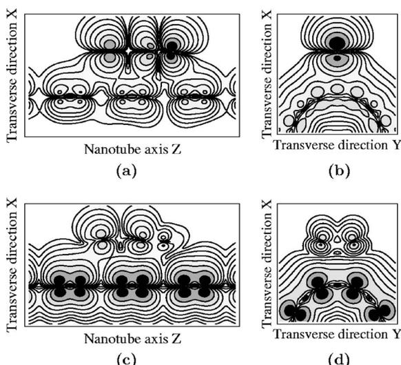
FIG. 6. Plots of charge density in five subbands at the top of the valence bands for [(a) and (b)]  $C_6H_5NH_2/SWNT(8,0)$  and [(c) and (d)]  $C_6H_5NO_2/SWNT(8,0)$ . In each figure the dark areas represent the highest densities. The contour plots are on a logarithmic scale. (a) and (c) show plots for the SWNT axial cuts; (b) and (d) show plots for cuts perpendicular to the SWNT axis through the functional atoms H for aniline and O for nitrobenzene.
