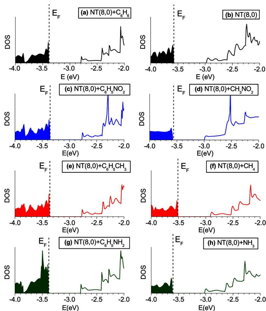
FIG. 4. (Color online) Total density of states for (a) benzene/SWNT (8,0), (b) clean/SWNT (8,0), (c) nitrobenzene/SWNT (8,0), (d) nitromethane/SWNT (8,0), (e) toluene/SWNT (8,0), (f) methane/SWNT (8,0), (g) aniline/SWNT (8,0), and (h)  $\text{NH}_3$ /SWNT (8,0).
