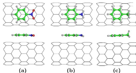
FIG. 2. (Color online) The lowest-energy configurations of simple benzene derivatives on SWNT(8,0): (a)  $C_6H_5NO_2$  near the top site, (b)  $C_6H_5NH_2$  near the bridge site, and (c)  $C_6H_5CH_3$  near the bridge site.
