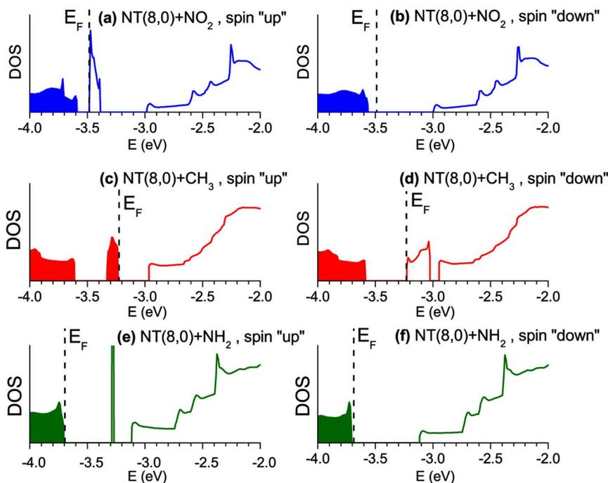
FIG. 5. (Color online) Total density of states from spin-polarized calculations for (a)  $\text{NO}_2/\text{SWNT}(8,0)$ , spin up; (b)  $\text{NO}_2/\text{SWNT}(8,0)$ , spin down; (c)  $\text{CH}_3/\text{SWNT}(8,0)$ , spin up; (d)  $\text{CH}_3/\text{SWNT}(8,0)$ , spin down; (e)  $\text{NH}_2/\text{SWNT}(8,0)$ , spin up; and (f)  $\text{NH}_2/\text{SWNT}(8,0)$ , spin up.
