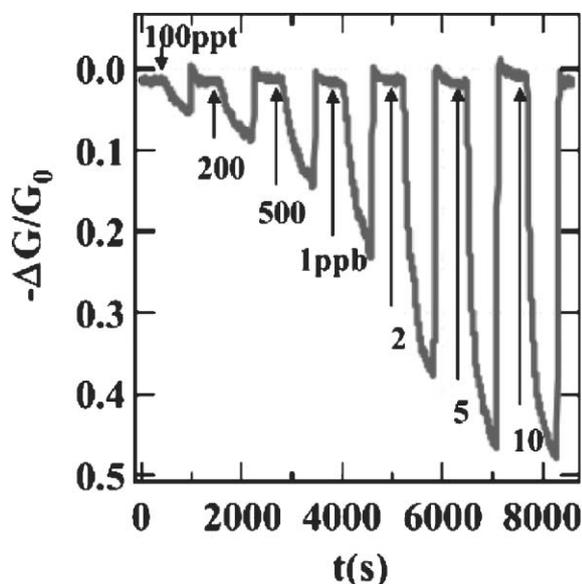
Fig. 4 Conductance response of a SWNT sensor to doses of NO<sub>2</sub> demonstrating 100-part-per-trillion sensitivity. The SWNTs were coated with PEI to enhance their sensitivity. The sensor was refreshed between doses by exposing it to ultraviolet light. (Reproduced with permission from Ref. 4. Copyright 2003 American Chemical Society.)
