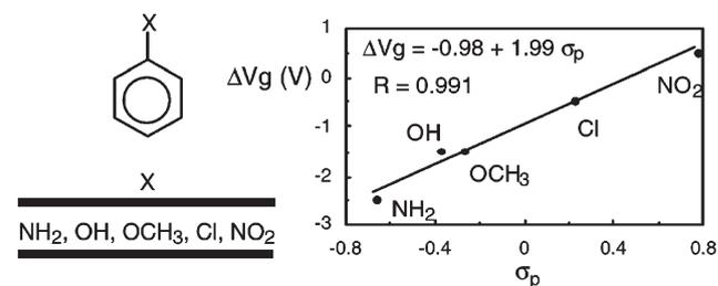
Fig. 5 Plot of the measured threshold shift (proportional to the amount of charge transfer) as a function of the Hammett constant,  $\sigma_p$ , of the benzene derivative. (Reproduced with permission from Ref. 20. Copyright 2003 American Chemical Society.)
