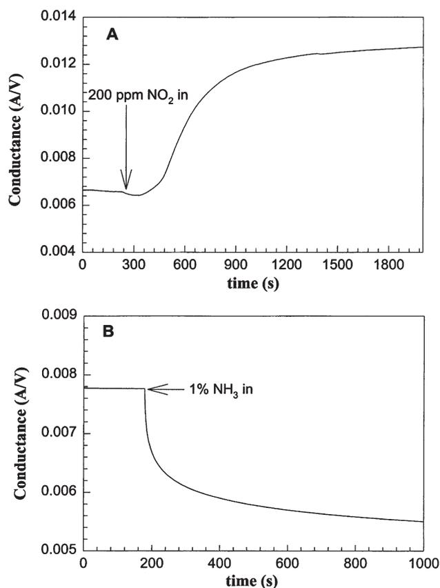
Fig. 3 Response of SWNTs to doses of NO<sub>2</sub> and NH<sub>3</sub>. (Reproduced with permission from Ref. 1. Copyright 2000 American Association for the Advancement of Science.)
