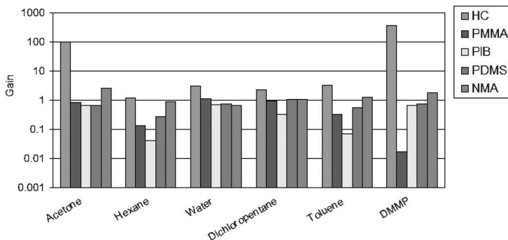
**Fig. 11** Ratio of the capacitance response of polymer-coated sensors to the response of an uncoated sensor for different vapors. The vapors were delivered at 0.01  $P_0$  except for DMMP which was delivered at 0.001  $P_0$ .
