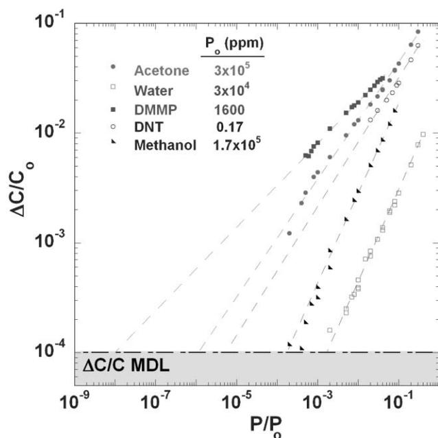
**Fig. 7** Capacitance response as a function of analyte concentration for different analytes. Each data set is well fit by the expression  $\Delta C/C = \alpha(P/P_0)^n$ , with  $n$  ranging from 0.4 to 1 and  $\alpha$  ranging from 0.01 to 0.2.  $P_0$  at room temperature for each analyte is listed in units of ppm.
