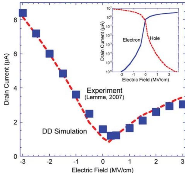
Fig. 6. Experimental data of [5], [6] and fit using a 1-D/2-D DD simulation, as discussed in the text. The inset shows the simulated electron and hole currents in the device.
