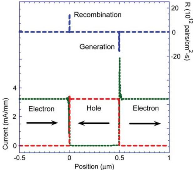
Fig. 8. Current and recombination rate as a function of source-drain bias in the FET simulated in Fig. 7 (no bandgap) and biased so that the channel is hole-rich ( $V_G = -1 \text{ V}$ ). Current flows are due to generation-recombination processes, particularly band-to-band tunneling.
