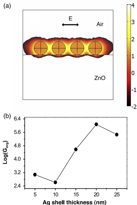
**Figure 4.** Simulations of log ( $G$ ) for silver particles with the size of 30 nm on a ZnO substrate. (a) The direction of the electric field polarization is shown by the double arrow. (b) The Ag shell thickness dependence of the average SERS of a 60 nm diameter ZnO nanowire.
