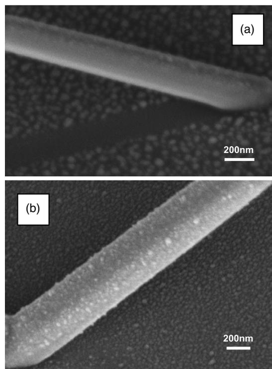
**Figure 2.** SEM images of e-beam (EB) deposited (a) and electroless (EL) plating (b) silver on ZnO NW, the angle between the incident electron beam and the sample stage is  $45^\circ$  for both (a) and (b).
