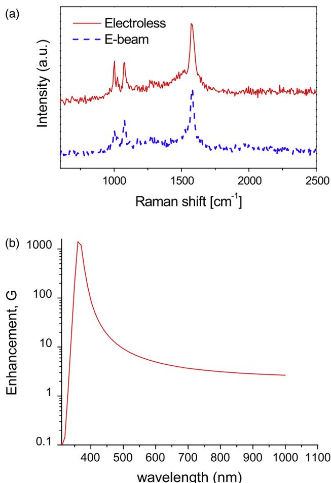
**Figure 3.** (a) Representative SERS on electroless (top solid curve) and E-beam (bottom dash curve) silver covered a single ZnO NW, and (b) surface plasmon resonance (SPR) simulation of 20 nm silver nanoparticles on ZnO NW.
