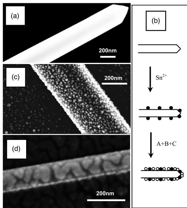
**Figure 1.** (a) SEM images of a bare nanowire as grown. (b) Schematic illustration of electroless (EL) silver plating on a single nanowire (A = silver ion solution, B = activator solution, C = reducer solution), (c) electroless (EL) Ag plated a single NW and (d) E-beam (EB) Ag evaporated a single NW.
