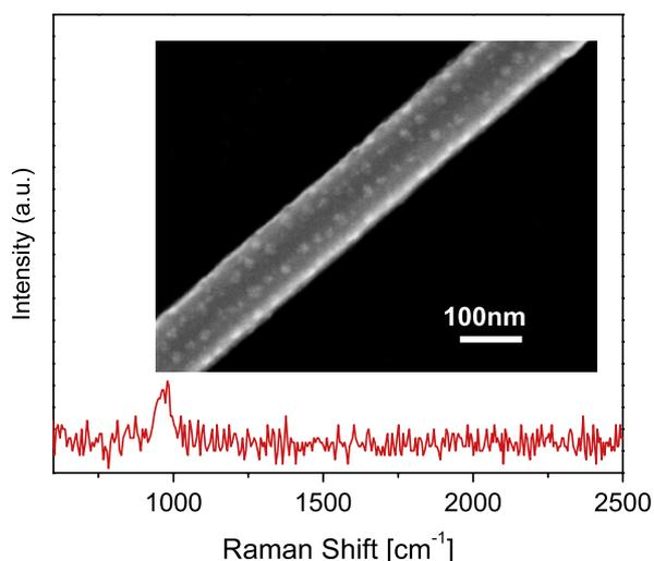
**Figure 5.** SERS measurement on a single nanowire with sparse silver nanoparticles, (inset) SEM image of a single nanowire with sparse silver nanoparticles produced via an electroless (EL) silver plating approach.
