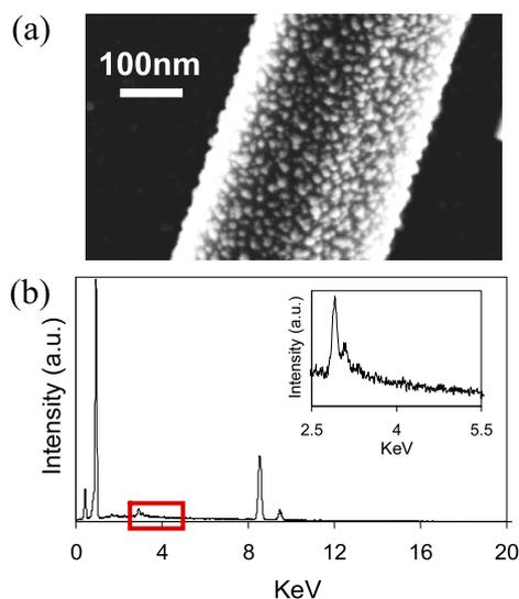
**Figure 1.** (a) SEM image of a dielectric ZnO NW core/Ag sheath composite produced by an electroless (EL) plating approach; (b) energy dispersive x-ray (EDX) spectra of the composites shown in (a); inset of (b) close-up plot of the silver EDX peak region (red rectangle).
