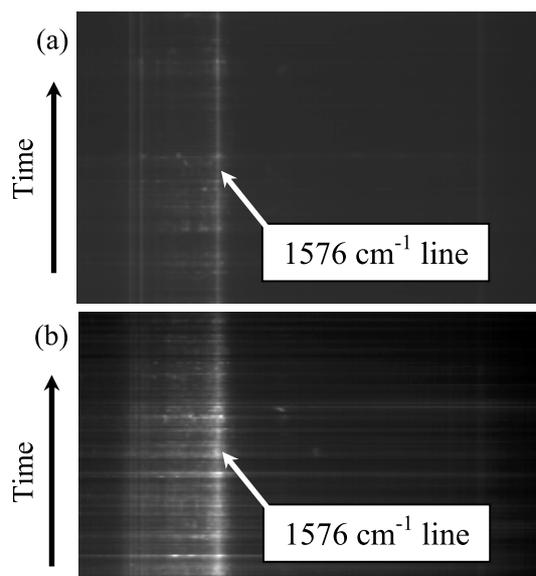
**Figure 3.** Time dependent behaviors of Ag on ZnO NW produced by (a) E-beam (EB), and (b) electroless (EL) depositions.
