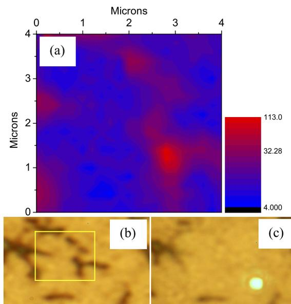
**Figure 4.** (a) Surface enhanced Raman spectroscopy (SERS) mapping of ZnO NWs core/silver sheath composites at the line of  $1576\text{ cm}^{-1}$ ; (b) and (c) microscope images before and after performing the mapping.
