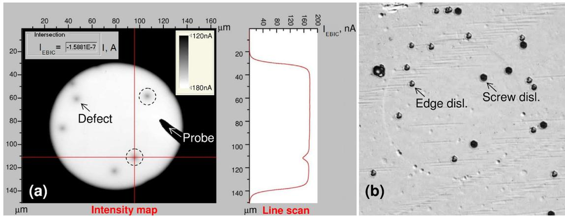
FIG. 2. (Color online) (a) EBIC intensity map acquired at 30 kV from a Schottky contact on an intentionally  $n$ -doped epilayer ( $1.1 \times 10^{16} \text{ cm}^{-3}$ ) and (b) corresponding Nomarski optical image after preferential molten KOH etching.
