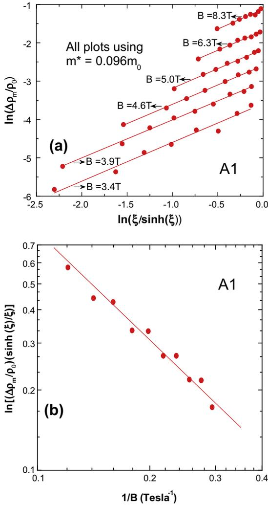
**Fig. 3.** (a) Effective hole mass is calculated using the temperature dependence of the oscillations as the value for which a gradient of unity is obtained in the plot of  $\ln(\frac{\Delta\rho_p}{\rho_0})$ , vs.  $\ln(\frac{\xi}{\sinh \xi})$ . (b) Dingle plot: Slope of line is  $-\pi\alpha/\mu$  where  $\alpha$  is the ratio  $\tau/\tau_q$  of the transport time  $\tau$  to the quantum lifetime  $\tau_q$ .
