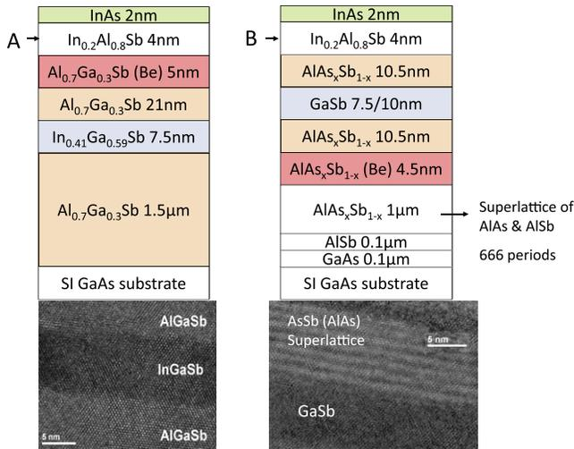
**Fig. 1.** Cross-section showing the layer details in a quantum well heterostructure with (A) In<sub>x</sub>Ga<sub>1-x</sub>Sb and (B) GaSb channel. The AlAs<sub>x</sub>Sb<sub>1-x</sub> layers are composed of AlSb/AlAs short-period superlattices. Also shown are high resolution TEM images around the channel region.
