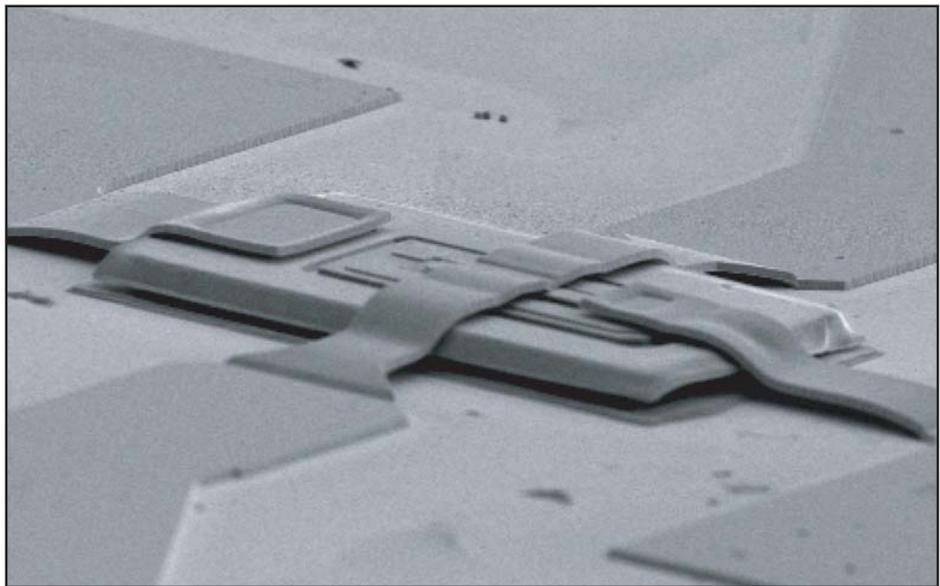
ABOVE: A scanning electron microscopy image of an InAlAsSb/InGaSb HBT fabricated in the 6.2 Å material system
