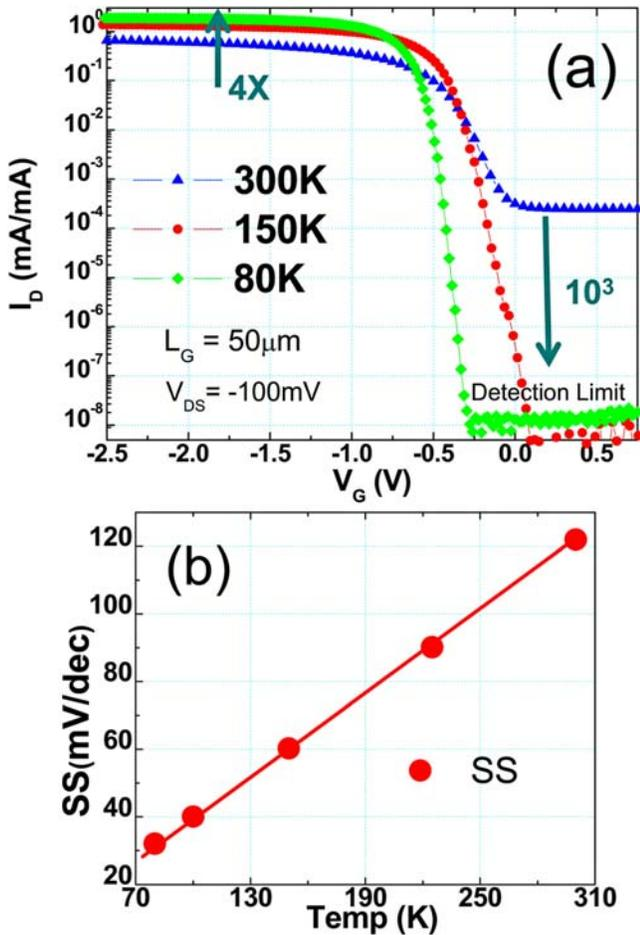
FIG. 11. (Color online) As the temperature is reduced from 300 K to 80 K: (a)  $I_{ON}$  increases by 4 times, while  $I_{OFF}$  decreases by 3 orders in magnitude; (b) the subthreshold swing (SS) decreases linearly as a function of temperature.
