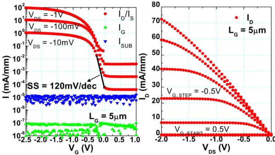
FIG. 6. (Color online)  $I_D$ - $V_G$  and  $I_D$ - $V_{DS}$  characteristics for surface channel  $In_{0.35}Ga_{0.65}Sb$  heterostructure MOSFET.  $I_{ON}/I_{OFF}$  is  $> 10^4$  and SS is 120 mV/decade.
