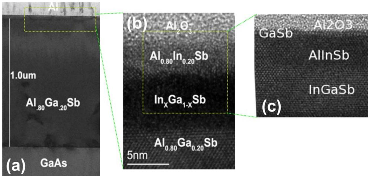
FIG. 4. (Color online) Cross section TEM on the buried  $\text{In}_x\text{Ga}_{1-x}\text{Sb}$  channel heterostructure MOSFET. (a)  $1.0 \mu\text{m}$  AlGaSb metamorphic buffer absorbs the lattice mismatch with the GaAs substrate. (b) Sharp interfaces between different layers and good crystal quality is maintained after device fabrication. (c) HRTEM shows sharp transition from amorphous oxide to crystalline semiconductor with 2 monolayers of GaSb intact at the semiconductor surface.
