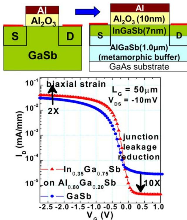
FIG. 5. (Color online) Comparing the  $I_D-V_G$  from bulk vs heterostructure design:  $I_{ON}$  is increased with the use of strain and confinement, while  $I_{OFF}$  is reduced by an order of magnitude due to reduction of body leakage from the drain contact.
