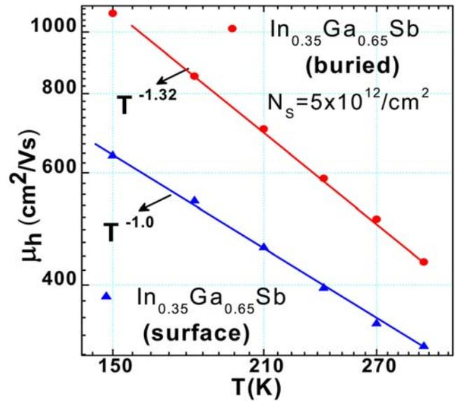
FIG. 13. (Color online) Hole mobility is plotted as a function of temperature at fixed sheet charge density of  $5 \times 10^{12}/\text{cm}^2$ . Temperature dependence of  $T^{-1}$  characteristic of mobility limited by interface scattering is observed for the surface channel design. The temperature dependence is  $T^{-1.32}$  for the buried channel design.
