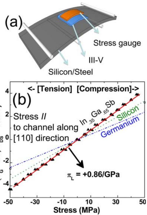
FIG. 9. (Color online) (a) Wafer bending setup used for studying the response of uniaxial strain. (b) 4.3% increase in current is observed with 50 MPa of uniaxial compression, corresponding to a piezoresistive coefficient ( $\pi_L$ ) of +0.86/GPa.
