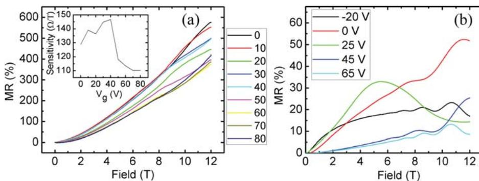
FIG. 2. (Color online) (a) MR for a typical shunted device showing a  $\sim 600\%$  change. The inset shows the sensitivity of the device. The slight oscillations are attributed to SdHO. (b) MR for a typical un-shunted device showing a much smaller change. The SdHO are much more pronounced.
