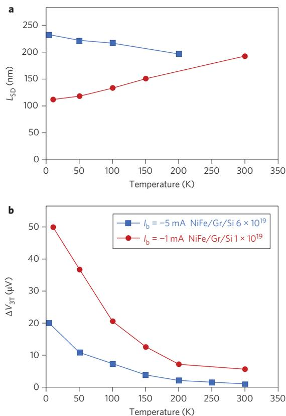
**Figure 5 | Temperature dependence of spin diffusion length and voltage.** **a**, Temperature dependence of  $L_{SD}$  is dominated by that of the diffusion constant. **b**, Measured three-terminal spin voltage decreases monotonically with increasing temperature.
