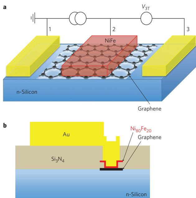
**Figure 1 | Schematic and cross-section of the samples.** **a**, Monolayer graphene serves as a tunnel barrier between the ferromagnetic metal contact and the Si substrate. Contacts 1 and 3 are ohmic Ti/Au contacts. **b**, The contact is designed so that the edges of the graphene are embedded in the SiN insulator, preventing conduction through the graphene edge states, which would short out the tunnel barrier.
