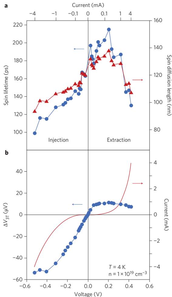
**Figure 4 | Bias dependence of spin lifetime/diffusion length and spin-voltage at 4 K. a**, Spin lifetime  $\tau_s$  and diffusion length  $L_{SD} = (D\tau_s)^{1/2}$  are at a maximum at low bias, and decrease with increasing positive and negative bias. **b**, Measured three-terminal spin voltage is strongly asymmetric with bias, although the conventional current-voltage characteristic is predominantly symmetric. The Si carrier concentration is  $n = 1 \times 10^{19} \text{ cm}^{-3}$ .
