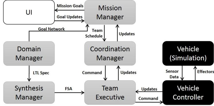
Fig. 4: A conceptual design of the Situated Decision Process (SDP). The Mission Manager performs Goal Reasoning operations. It creates a schedule of actions for a team of vehicles, each of which operates a synthesized Finite State Automaton.
