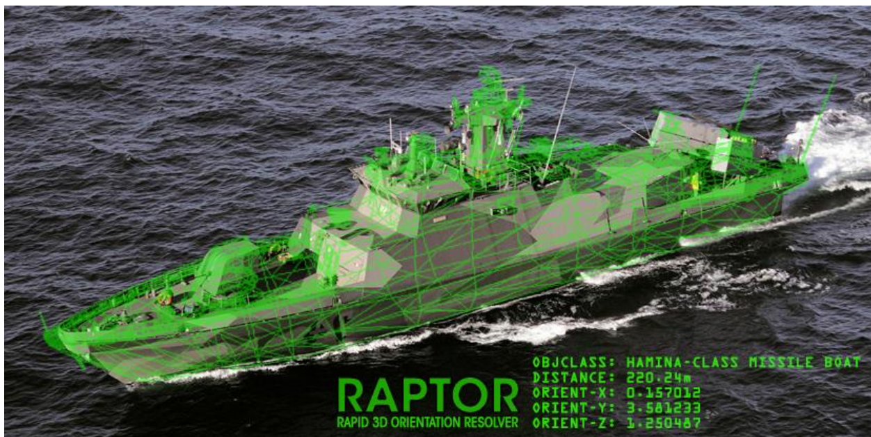
Figure 1.1: A properly oriented 3D mesh of a Hamina-class missile boat shown superimposed over a real-world picture of said boat. Since the 3D model is properly oriented with respect to the picture, we can easily calculate non-trivial state information, such as movement speed, trajectory, potential collisions with and proximity to other objects, etc. The goal of RAPTOR is to be able to estimate object poses like this on the fly in a highly accurate, real-time fashion.
