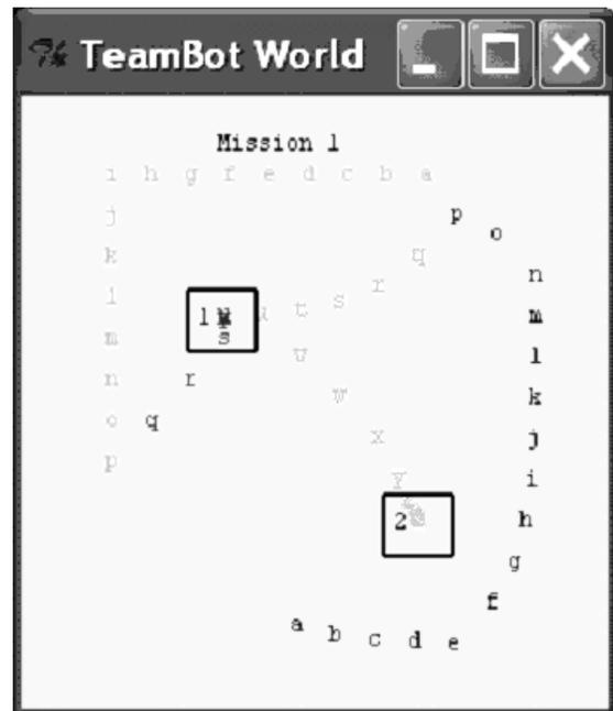
Figure 3. Track of the human (starting at top) and TeamBot (starting at the bottom) 'manning' two guard stations (numbered squares) with a conflict. Both began at their respective "a" locations and patrolled counter-clockwise until the alarm occurred at "p." Then both moved toward guard station #1 until, at step "u," the TeamBot detects the conflict and goes to station #2.
