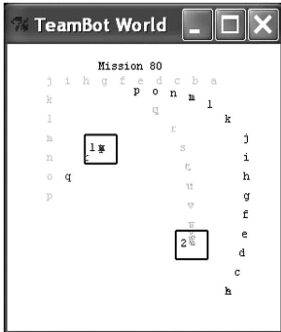
Figure 4. Track of the human (starting at top) and TeamBot (starting at the bottom) avoiding a conflict by simulating the human’s decision making. Both began at their respective (a) locations and patrolled counter-clockwise until the alarm occurred at (p). The TeamBot then, in accordance with the shared plan, determined where the human would go by simulating the human’s decision-making using its own knowledge and therefore immediately started toward the other station.
