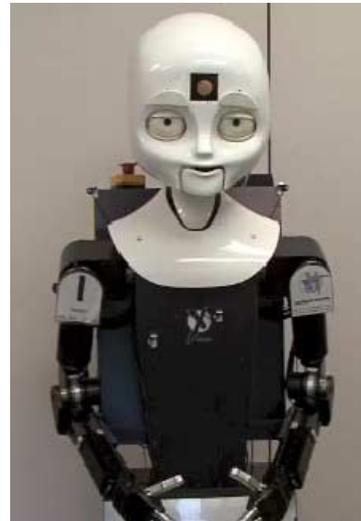
Figure 2: Octavia in neutral position in Voice condition: head up, eyes open and alert, arms and hands in a non-threatening position, body and head facing the audience.
