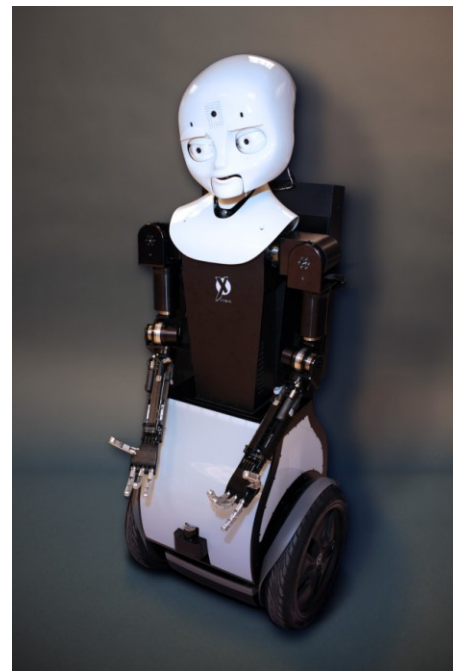
Fig1. Octavia is an MDS robot with a 4-element microphone array mounted on the body and cameras in the eyes.
