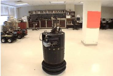
**Figure 2: The robot turning 180 degrees to "close" its eyes.**
