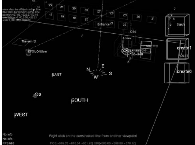
Figure 4. Lines intersection technique. Here two users (the current user’s position is denoted by the compass rose at the center of the screen, the remote user’s avatar is shown as the light gray box with the label “EP-SILONUser”) are shooting rays in the environment by pointing a common point on the real world (not shown here). The result is that the point they identified (bottom right corner of window 27) is created in 3D. Note that a single user could do this operation from two different viewpoints.
