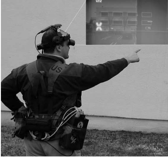
Figure 1. The BARS mobile augmented reality system. On the right of the user is the computer. The HMD is equipped with a GPS antenna and a USB camera. The insert shows an image which was taken by a camera placed at the eye piece of the head mounted display.
